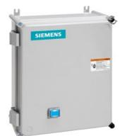
Non-reversing motor starter, Size 1, Single phase full voltage, Solid-state overload relay, OLR amp range 0.75-3.4A, Non-combination type, Enclosure type 4X fiberglass, Water/dust tight noncorrosive, Standard width enclosure
