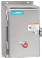
Non-reversing motor starter Size 1 Three phase full voltage Solid-state overload relay OLRelay amp range 0.25-1A 110VAC 50HZ / 120VAC 60HZ coil Combination type Water/dust tight non-corrosive
