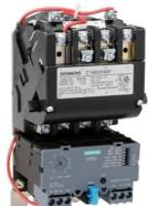
Non-reversing motor starter Size 1 Three phase full voltage Solid-state overload relay OLRelay amp range 0.25-1A 240VAC 50HZ / 277VAC 60HZ coil Combination type No enclosure
