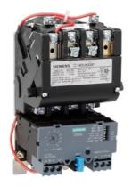
Non-reversing motor starter Size 1 Three phase full voltage Solid-state overload relay OLRelay amp range 0.25-1A 380-440/440-480V 50/60HZ coil Combination type No enclosure
