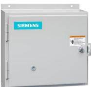
Non-reversing motor starter, Size 1, Three phase full voltage, Solid-state overload relay, OLRelay amp range 0.25-1a, 240V 50HZ / 277V 60HZ coil, Non-combination type, Enclosure type 12, Dust/drip proof for indoors, Standard width enclosure
