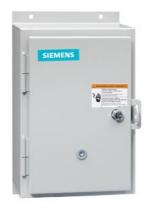
Non-reversing motor starter, Size 0, Three phase full voltage, Solid-state overload relay, OLRelay amp range 5.5-22a, 550/575 600 50/60HZ coil, Non-combination type, Enclosure type 12, Dust/drip proof for indoors, Extra-wide enclosure
