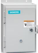
Non-reversing motor starter, Size 0, Three phase full voltage, Solid-state overload relay, OLRelay amp range 5.5-22a, 220 240/440 480VAC 60HZ coil, Non-combination type, Enclosure type 12, Dust/drip proof for indoors, Extra-wide enclosure
