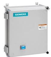
Non-reversing motor starter, Size 0, Three phase full voltage, Solid-state overload relay, OLR amp range 5.5-22A, 208VAC 60Hz coil, Non-combination type, Enclosure type 4X fiberglass, Water/dust tight noncorrosive, Standard width enclosure
