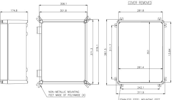
STAINLESS STEEL MOUNTING FEET MOUNTED VERTICAL OR HORIZONTAL
