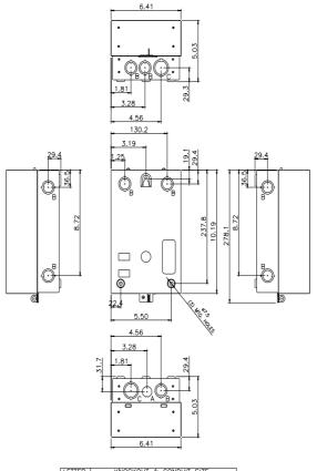
KNOCKOUT & CONDUIT SIZE @22.2 FOR 12.7 CONDUIT @22.2 X @28.6 FOR 12.7 & 19 CONDUIT @28.6 X @34.9 FOR 19 & 25.4 CONDUIT
