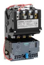
Non-reversing motor starter Size 0 Three phase full voltage Solid-state overload relay OLRelay amp range 5.5-22A 240VAC 50HZ / 277VAC 60HZ coil Combination type No enclosure
