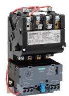
Non-reversing motor starter Size 0 Three phase full voltage Solid-state overload relay OLRelay amp range 5.5-22A 24VAC 50-60HZ coil Combination type No enclosure
