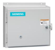
Non-reversing motor starter, Size 0, Three phase full voltage, Solid-state overload relay, OLR amp range 5.5-22A, Non-combination type, Enclosure type 12, Dust/drip proof for indoors, Standard width enclosure
