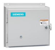
Non-reversing motor starter, Size 0, Three phase full voltage, Solid-state overload relay, OLR amp range 3-12A, 240V 50Hz / 277V 60Hz coil, Non-combination type, Enclosure type 12, Dust/drip proof for indoors, Standard width enclosure
