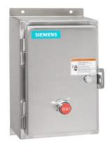
Non-reversing motor starter, Size 0, Single phase full voltage, Solid-state overload relay, OLR amp range 3-12A, 110V 50Hz / 120V 60Hz coil, Non-combination type, Encl. type 4X 304 S. Steel, Water/dust tight noncorrosive, Standard width
