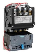
Non-reversing motor starter Size 0 Single phase full voltage Solid-state overload relay OLRelay amp range 3-12A 208VAC 60HZ coil Combination type No enclosure
