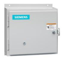
Non-reversing motor starter, Size 0, Single phase full voltage, Solid-state overload relay, OLR amp range 3-12A, 110V 50Hz / 120V 60Hz coil, Non-combination type, Enclosure type 12, Dust/drip proof for indoors, Standard width enclosure
