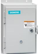
Non-reversing motor starter, Size 0, Three phase full voltage, Solid-state overload relay, OLRelay amp range 0.75-3.4a, 220 240/440 480VAC 60HZ coil, Non-combination type, Enclosure type 12, Dust/drip proof for indoors, Extra-wide enclosure
