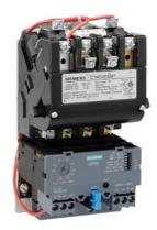
Non-reversing motor starter Size 0 Three phase full voltage Solid-state overload relay OLRelay amp range 0.75-3.4A 208VAC 60HZ coil Combination type No enclosure
