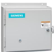
Non-reversing motor starter, Size 0, Three phase full voltage, Solid-state overload relay, OLR amp range 0.75-3.4A, 110V 50Hz / 120V 60Hz coil, Non-combination type, Enclosure type 12, Dust/drip proof for indoors, Standard width enclosure
