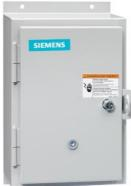
Non-reversing motor starter, Size 0, Three phase full voltage, Solid-state overload relay, OLRelay amp range 0.25-1a, 240V 50HZ / 277V 60HZ coil, Non-combination type, Enclosure type 12, Dust/drip proof for indoors, Extra-wide enclosure
