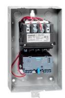
Non-reversing motor starter, Size 00, Three phase full voltage, Solid-state overload relay, OLR amp range 3-12A, Non-combination type, Enclosure type 1, Indoor general purpose use, Standard width enclosure
