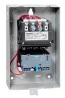
Non-reversing motor starter Size 00 Three phase full voltage Solid-state overload relay OLRelay amp range 0.25-1A 220-240/440-480VAC 60HZ coil Combination type Indoor general purpose use
