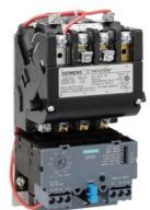
Non-reversing motor starter Size 00 Three phase full voltage Solid-state overload relay OLRelay amp range 0.25-1A 110VAC 50HZ / 120VAC 60HZ coil Combination type No enclosure
