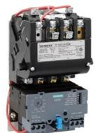
Non-reversing motor starter Size 00 Three phase full voltage Solid-state overload relay OLRelay amp range 0.25-1A 220-240/440-480VAC 60HZ coil Combination type No enclosure
