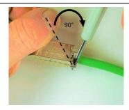
**K**. Insert a 2.5 mm screw driver into the hole of locking part and turn it as far as limit stop.
