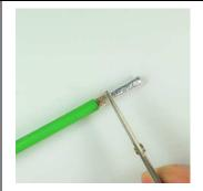
F. Pull-out the outer jacket material & remove the protective foil and unwanted braid bristle with scissors and keep it smooth
