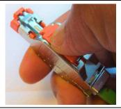
L. Unmate the connector by pressing the button with thumb (refer **M** for an alternative)
