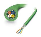
Data cable, PROFINET CAT5 (100 Mbps), 4-position, PVC/PVC, green RAL 6018, shielded (Aluminum-coated foil, tinned copper braided shield), free cable end, on free cable end, cable length: 100 m
