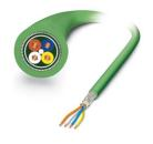
Data cable, PROFINET CAT5 (100 Mbps), 4-position, PVC/PVC, green RAL 6018, shielded (Aluminum-coated foil, tinned copper braided shield), free cable end, on free cable end, cable length: Free entry (0.5 ... 400 m)
