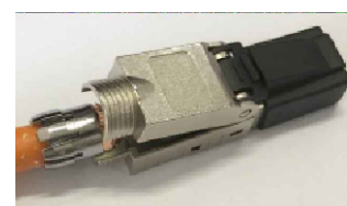
8.Press the shielded cover to jack.Make secure contact with cable.
