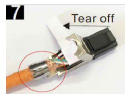
7.Put the termination cap onto the IDC Part &amp; Tear off the color code paper. Make the termination cap on the right way.
