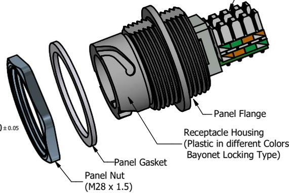
Shielded Cat.5e RJ45 IDC Jack accepts both Solid and Stranded AWG 24 to 26 Wires
