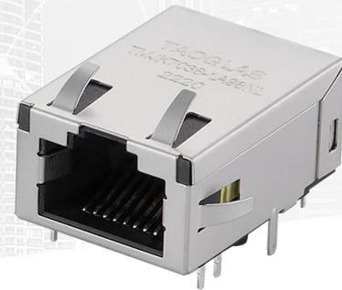
Featuring a popular footprint and compatible package to industry RJ45 Integrated Connectors standards, the Taoglas TMJK7036-1A98NL is an RJ45 Integrated Connector 1G Base-T Single Port Tab Up with EMI Finger and 3Wire Common Mode Choke on the chip side that enables AutoMDIX feature.
