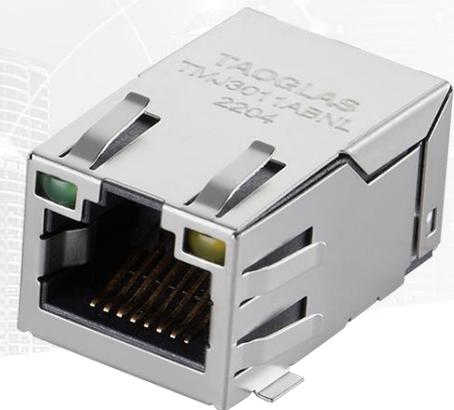
Featuring a popular footprint and compatible package to industry RJ45 Integrated Connectors standards, the Taoglas TMJ3011ABNL is an RJ45 Integrated Connector 10/100Base-T Single Port Tab Up with EMI Finger, its shielded body design offers extra space, and with a schematic that enables AutoMDIX feature.
