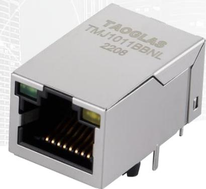
Featuring a popular footprint and compatible package to industry RJ45 Integrated Connectors standards, the Taoglas TMJ1011BBNL is an RJ45 Integrated Connector 10/100Base-T Single Port Tab Up with shielded body and with a schematic that enables AutoMDIX feature.
