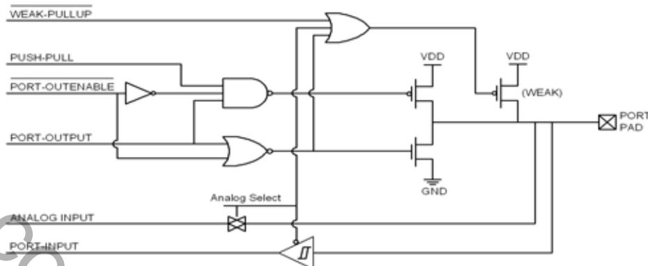
Figure 20.2. Port I/O Cell Block Diagram
