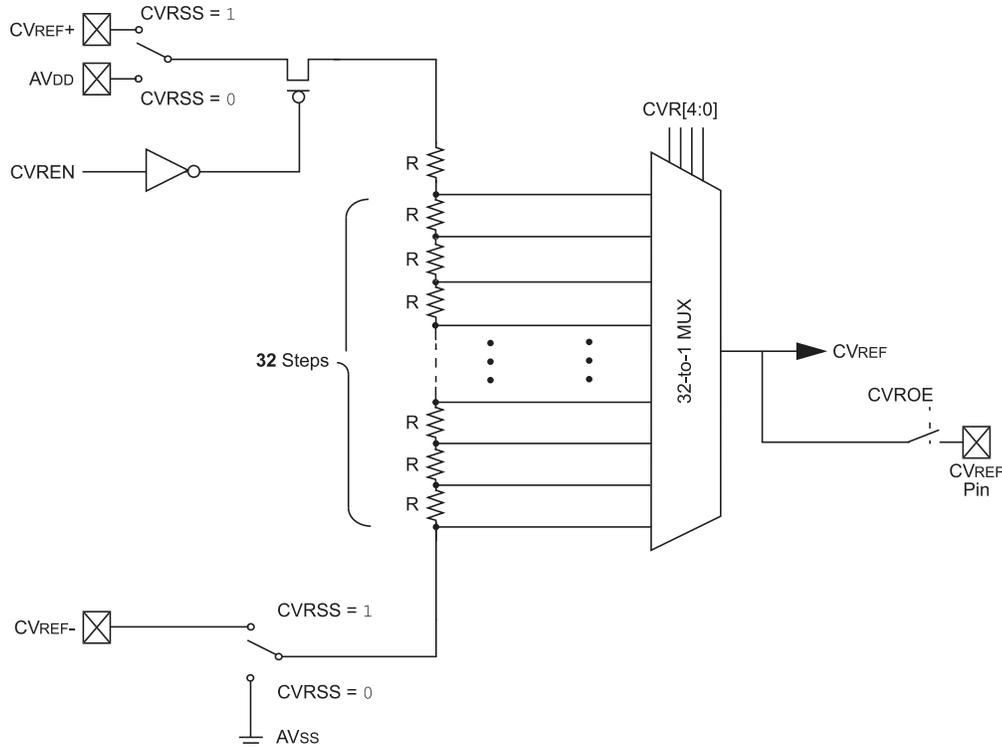
The voltage reference module is controlled through the CVRCON register. The comparator voltage reference provides two ranges of output voltage, each with 16 distinct levels. The primary difference between the ranges is the size of the steps selected by the CV<sub>REF</sub> Value Selection bits (CVR[4:0]), with one range offering finer resolution.
