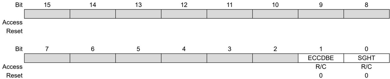
**Bit 1 – ECCDBE** ECC Double-Bit Error Trap bit
