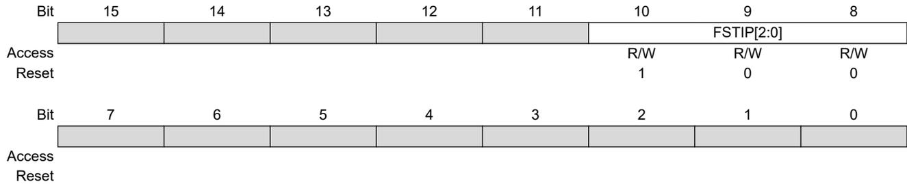
**Bits 10:8 – FSTIP[2:0]** FRC Self-Tuning Interrupt Priority bits
