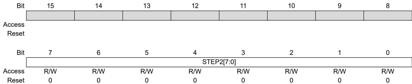
**Bits 7:0 – STEP2[7:0]** DMT Clear Enable bits
