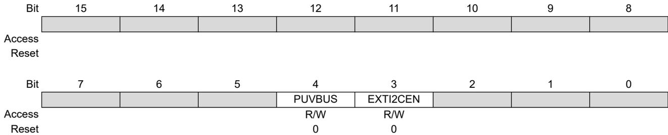
**Bit 4 – PUVBUS**  $V_{BUS}$  Pull-up Enable bit
