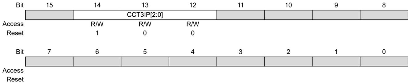
**Bits 14:12 – CCT3IP[2:0]** Capture/Compare/Timer3 Interrupt Priority bits
