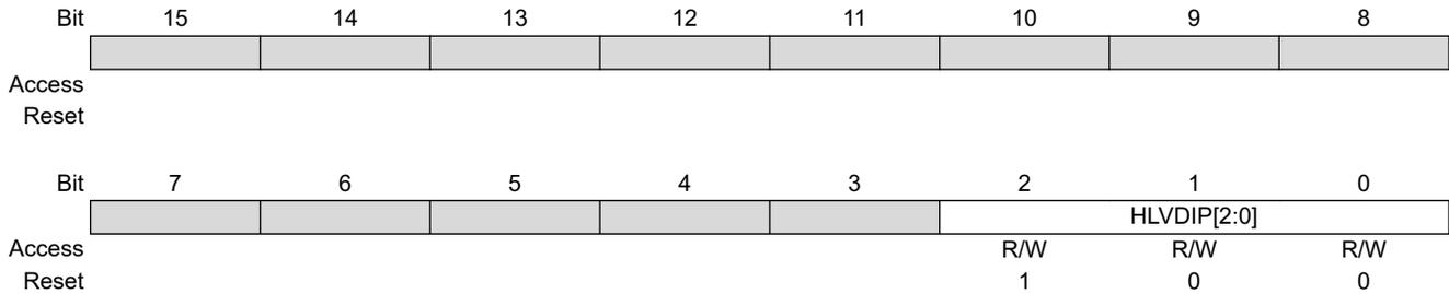
**Bits 2:0 – HLVDIP[2:0]** High/Low-Voltage Detect Interrupt Priority bits
