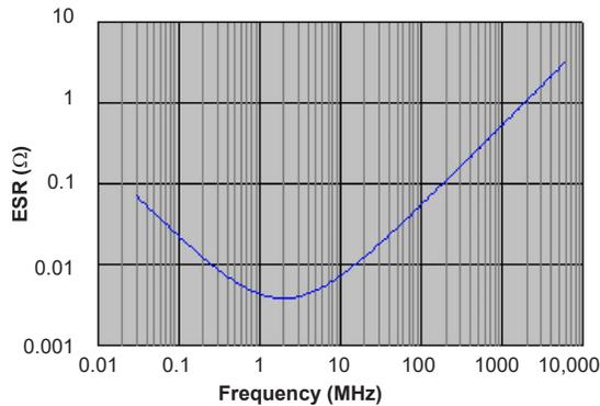
**Note:** Typical data measurement at  $+25^\circ\text{C}$ , 0V DC bias.
