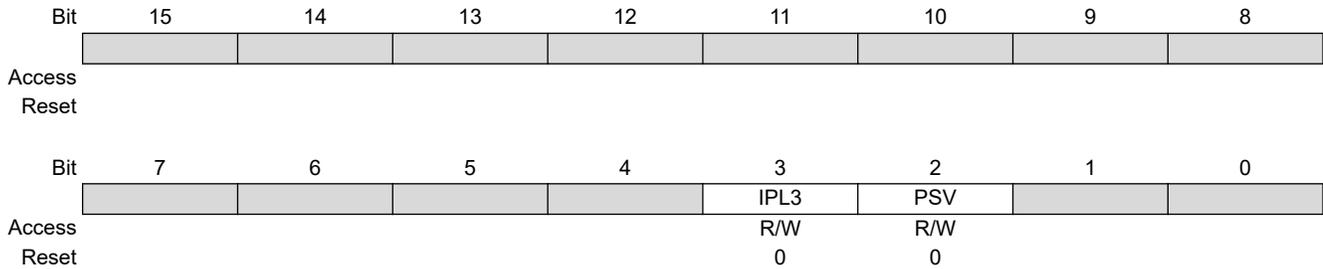
**Bit 3 – IPL3** CPU Interrupt Priority Level Status bit<sup>(1)</sup>
