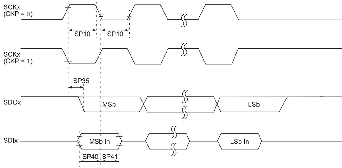
Figure 30-10. SPI Module Host Mode (CKE = 1) Timing Characteristics
