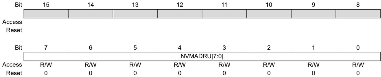
**Bits 7:0 – NVMADRU[7:0]** Nonvolatile Memory Write Address Upper bits
