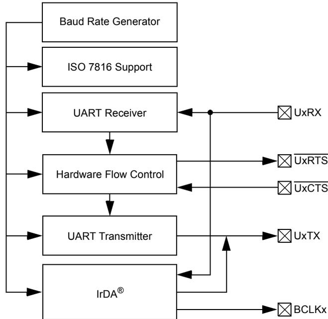
**Note:** The UART inputs and outputs must all be assigned to available RPN/RPIn pins before use. See [11.4 Peripheral Pin Select \(PPS\)](#) for more information.
