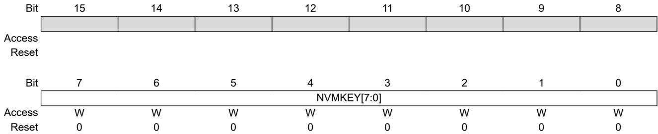
**Bits 7:0 – NVMKEY[7:0]** NVM Key Register bits (write-only)
