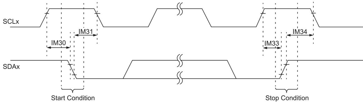
**Figure 30-14. I<sup>2</sup>C Bus Data Timing Characteristics (Host Mode)**
