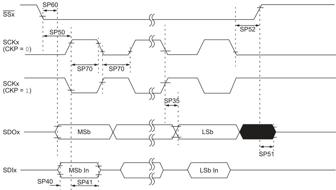
**Table 30-26. SPI Module Client Mode Timing Requirements**
