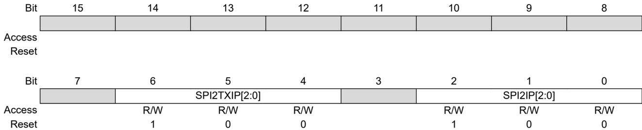
**Bits 6:4 – SPI2TXIP[2:0]** SPI2 Transfer Done Interrupt Priority bits
