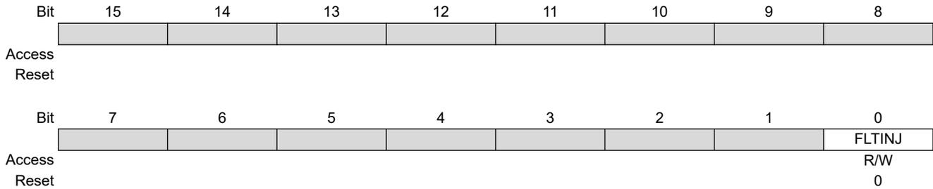
**Bit 0 – FLTINJ** Fault Injection Sequence Enable bit
