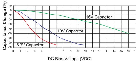
When selecting a ceramic capacitor to be used with the internal voltage regulator, it is suggested to select a high-voltage rating so that the operating voltage is a small percentage of the maximum rated capacitor voltage. For example, choose a ceramic capacitor rated at a minimum of 16V for the 1.8V core voltage. Suggested capacitors are shown in [Table 2-1](#).
