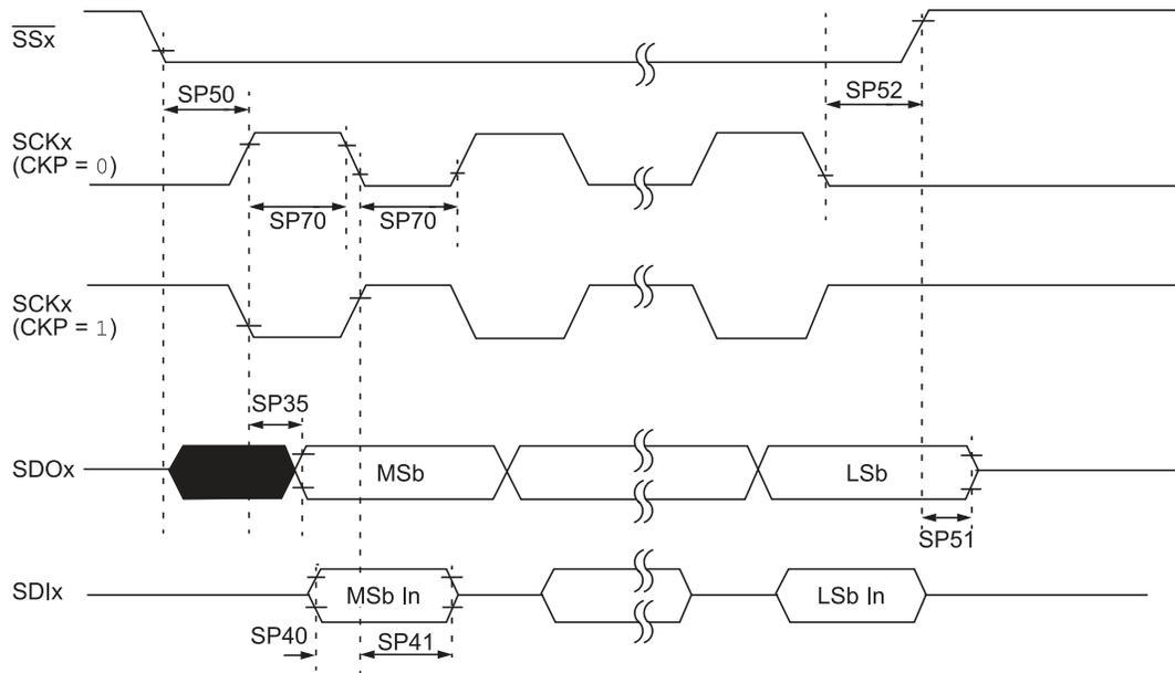
**Figure 30-12. SPI Module Client Mode (CKE = 1) Timing Characteristics**
