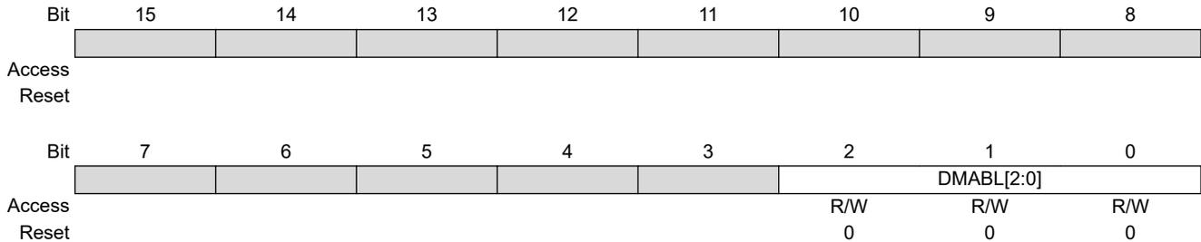
**Bits 2:0 – DMABL[2:0]** DMA Buffer Size Select bits<sup>(1)</sup>
