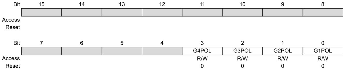
**Bit 3 – G4POL** Gate 4 Polarity Control bit
