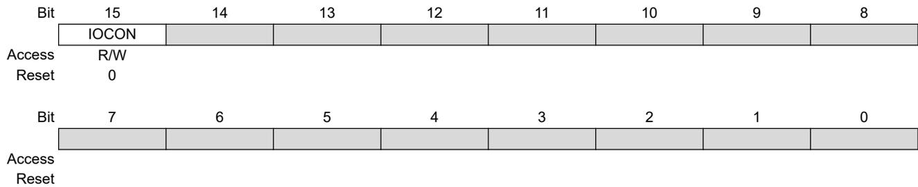
**Bit 15 – IOCON** Interrupt-on-Change Enable bit
