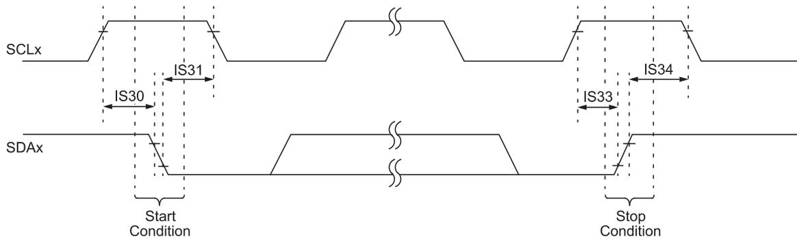
**Figure 30-16. I<sup>2</sup>C Bus Data Timing Characteristics (Client Mode)**
