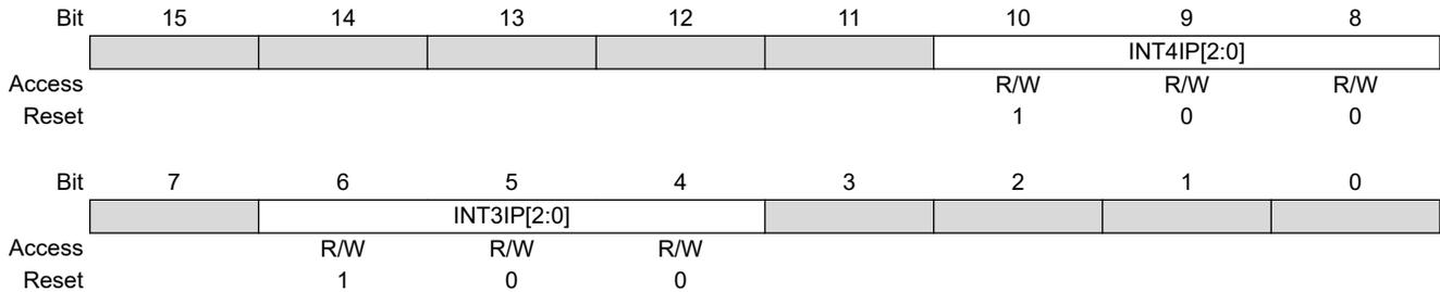
**Bits 10:8 – INT4IP[2:0]** External Interrupt 4 Interrupt Priority bits
