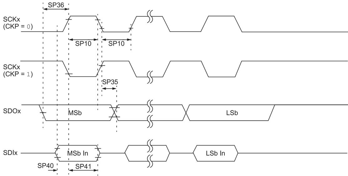
**Table 30-25. SPI Module Host Mode Timing Requirements**
