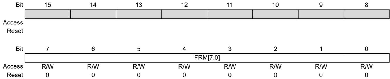
**Bits 7:0 – FRM[7:0]** Data Frame Counter bits
