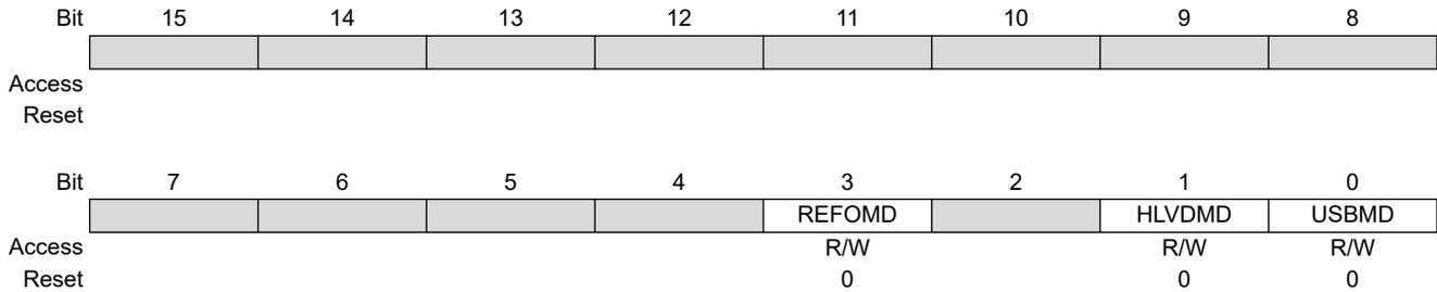
**Bit 3 – REFOMD** Reference Clock Output Module Disable bit
