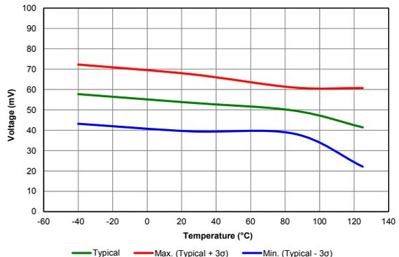
Figure 39-18. BROWN-OUT RESET VOLTAGE, TRIP POINT (BORV = 11)
