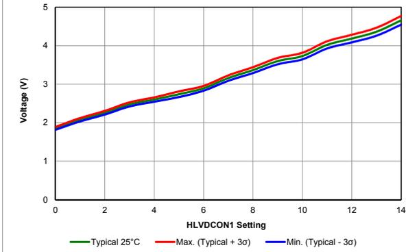
Figure 39-61. LVD Comparator Output Low Trip Points
