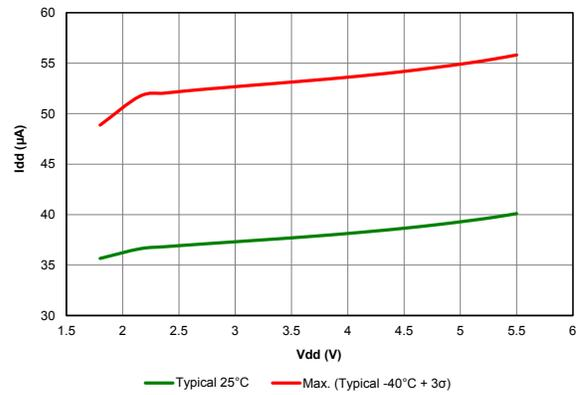
Figure 39-47. I<sub>PD</sub>, WATCH DOG TIMER (WDT)
