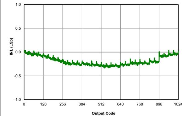
Figure 39-6. ADC, INL, Vdd = 3.0V, TAD = 4uS, 25C
