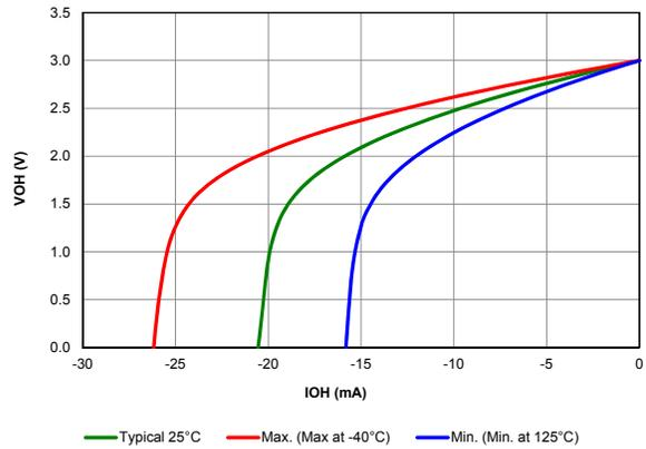
Figure 39-78. VOH vs. IOH OVER TEMPERATURE, VDD = 1.8V
