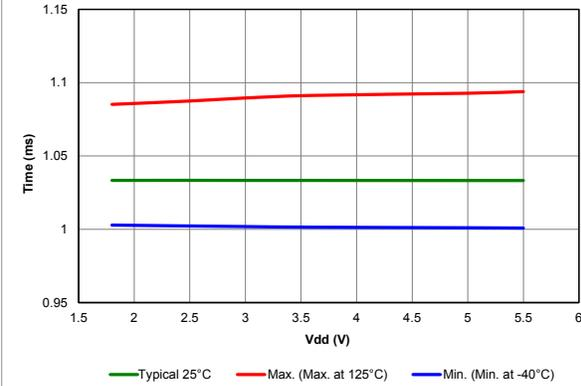
**Figure 39-83. WDT BASE TIME-OUT PERIOD (WDTPS = 0, V<sub>DD</sub> = 3.0V)**
