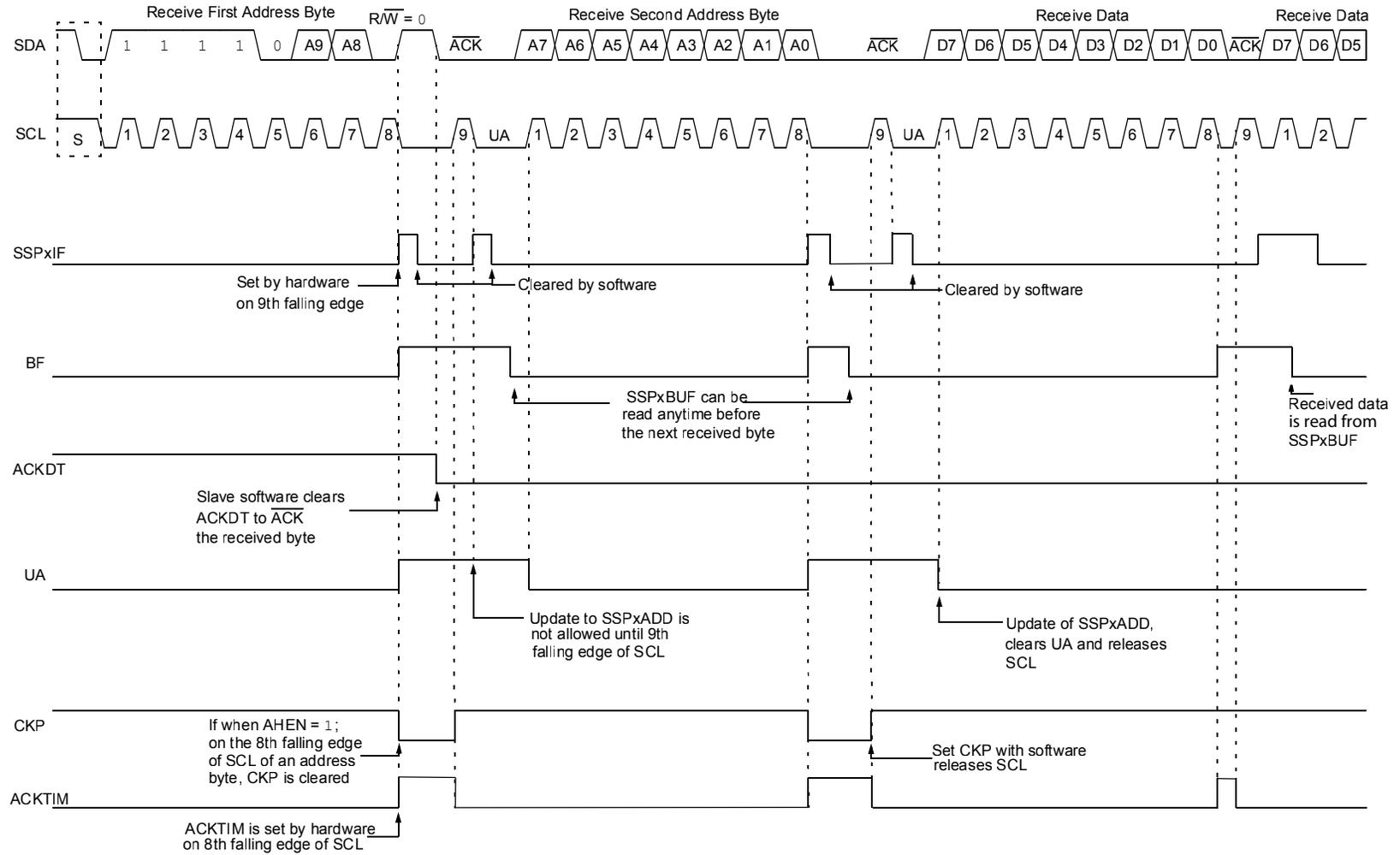
Figure 26-22. I<sup>2</sup>C Slave, 10-bit Address, Transmission (SEN = 0, AHEN = 0, DHEN = 0)
