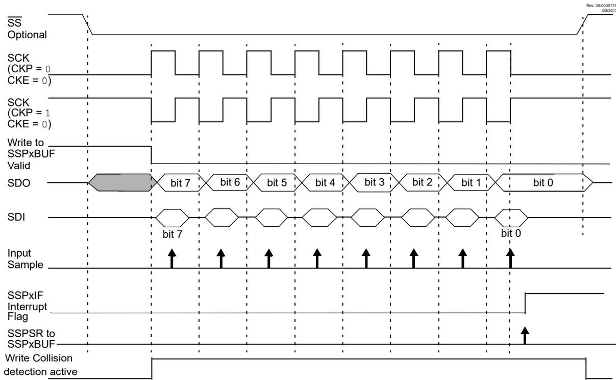
Figure 26-8. SPI Mode Waveform (Slave Mode with CKE = 1)
