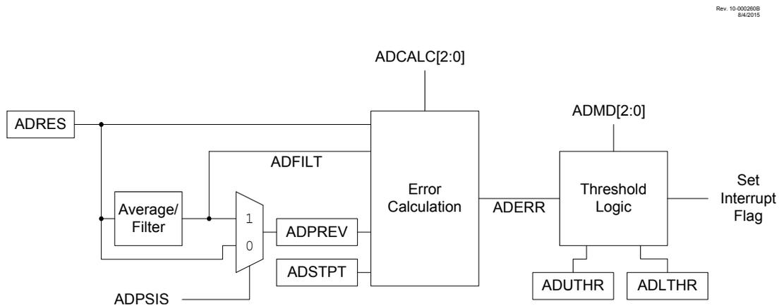
The operation of the ADC computational features is controlled by the ADMD bits.
