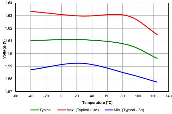
Figure 39-64. POR RELEASE VOLTAGE, (VREGPM =  $\text{'b0x}$ )
