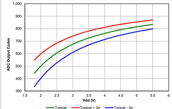
**Figure 39-70. TEMPERATURE INDICATOR SLOPE NORMALIZED TO 20°C, HIGH RANGE,  $V_{DD} = 5.5V$**
