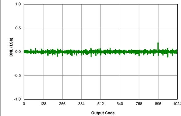
Figure 39-4. ADC, DNL, Vdd = 3.0V, TAD = 4uS, 25C
