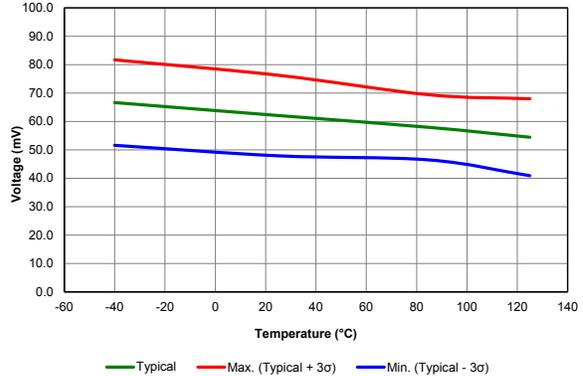
Figure 39-14. BROWN-OUT RESET VOLTAGE, TRIP POINT (BORV = 01)
