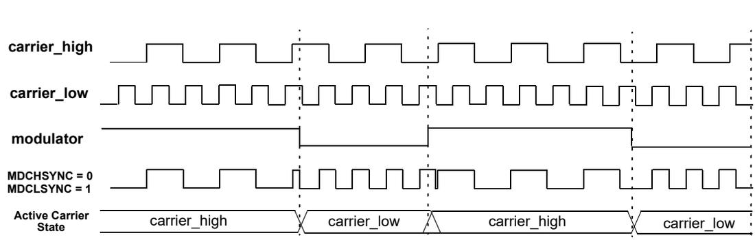
**Figure 25-6. Full Synchronization (MDCHSYNC = 1, MDCLSYNC = 1)**
