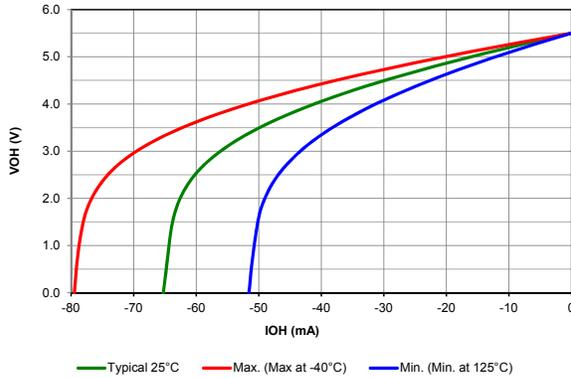
Figure 39-77. VOH vs. IOH OVER TEMPERATURE, VDD = 3V
