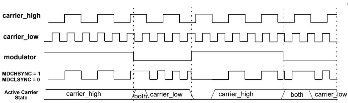
**Figure 25-5. Carrier Low Synchronization (MDCHSYNC = 0, MDCLSYNC = 1)**
