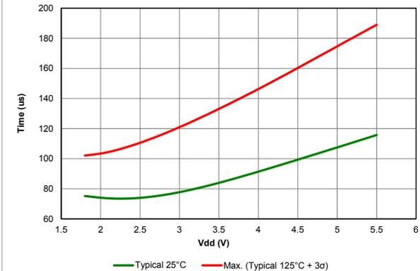
Figure 39-54. Wake From Sleep, VREGPM = 'b0x, HFINTOSC = 16MHz
