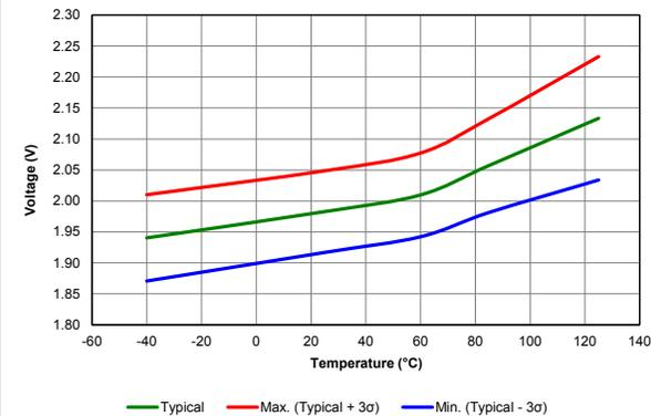
Figure 39-58. LOW POWER BROWN-OUT RESET REARM VOLTAGE
