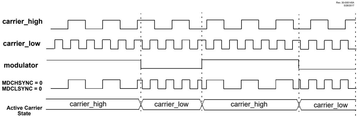
**Figure 25-4. Carrier High Synchronization (MDCHSYNC = 1, MDCLSYNC = 0)**
