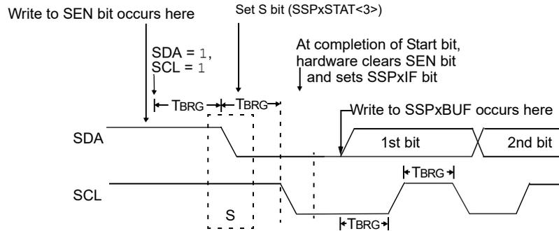
**26.6.5 I<sup>2</sup>C Master Mode Repeated Start Condition Timing**
