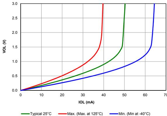
Figure 39-81. VOL vs. IOL OVER TEMPERATURE, VDD = 1.8V
