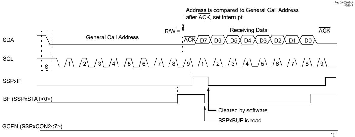
In 10-bit Address mode, the UA bit will not be set on the reception of the general call address. The slave will prepare to receive the second byte as data, just as it would in 7-bit mode.
