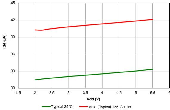
Figure 39-46. I<sub>PD</sub>, COMPARATOR
