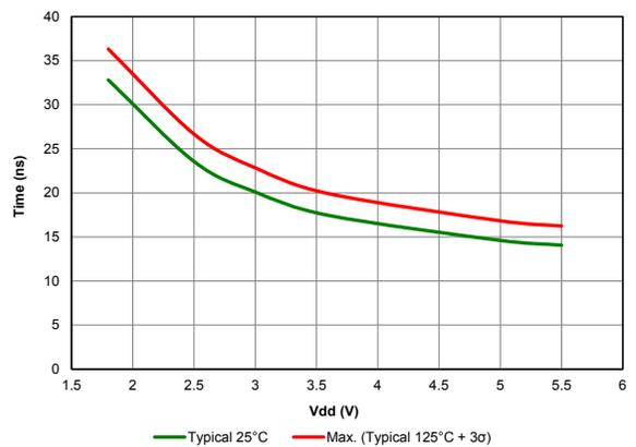
Figure 39-34. Rise time, slew rate control disabled
