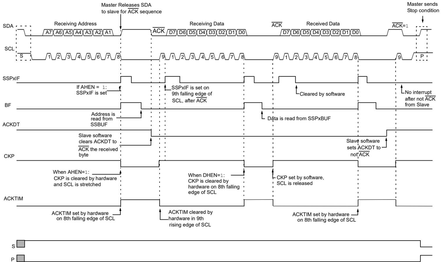
Figure 26-17. I<sup>2</sup>C Slave, 7-bit Address, Reception (SEN = 1, AHEN = 1, DHEN = 1)
