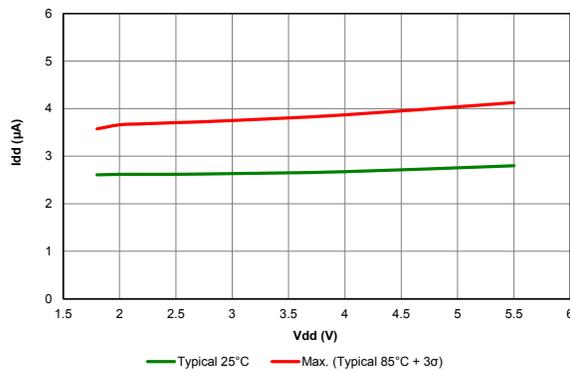
Figure 39-37. I<sub>DD</sub> TYPICAL, INT Oscillator
