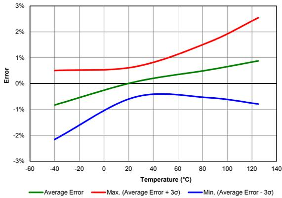
Figure 39-30. FVR Voltage Error 2x (Vdd = 5.5 V)
