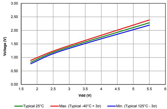
Figure 39-44. TTL Input Level
