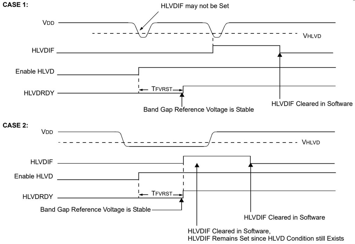
**Figure 33-3. High-Voltage Detect Operation (INTH = 1)**
