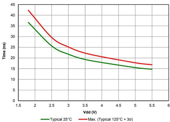
Figure 39-33. Fall time, slew rate control enabled
