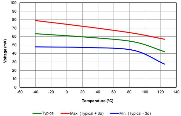
Figure 39-16. BROWN-OUT RESET VOLTAGE, TRIP POINT (BORV = 10)
