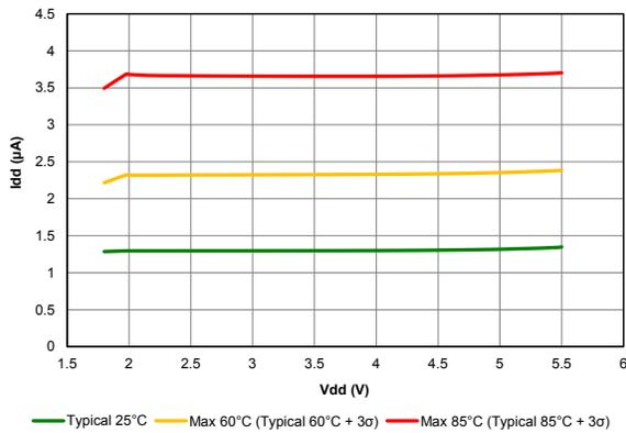
Figure 39-48. I<sub>PD</sub>, FIXED VOLTAGE REFERENCE (FVR)
