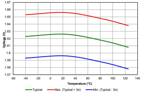
Figure 39-65. POR REARM VOLTAGE, (VREGPM =  $\text{'b1x}$ )
