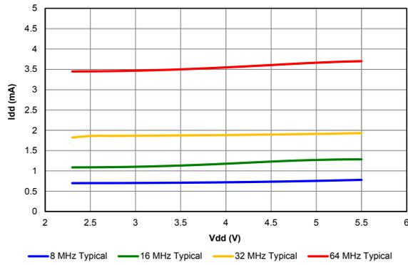
Figure 39-41.  $I_{DD}$ , ECH OSCILLATOR, MAXIMUM
