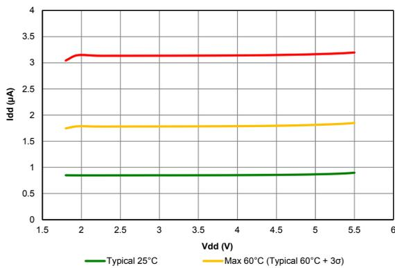
Figure 39-50. I<sub>PD</sub> BASE (VREGPM='b01)
