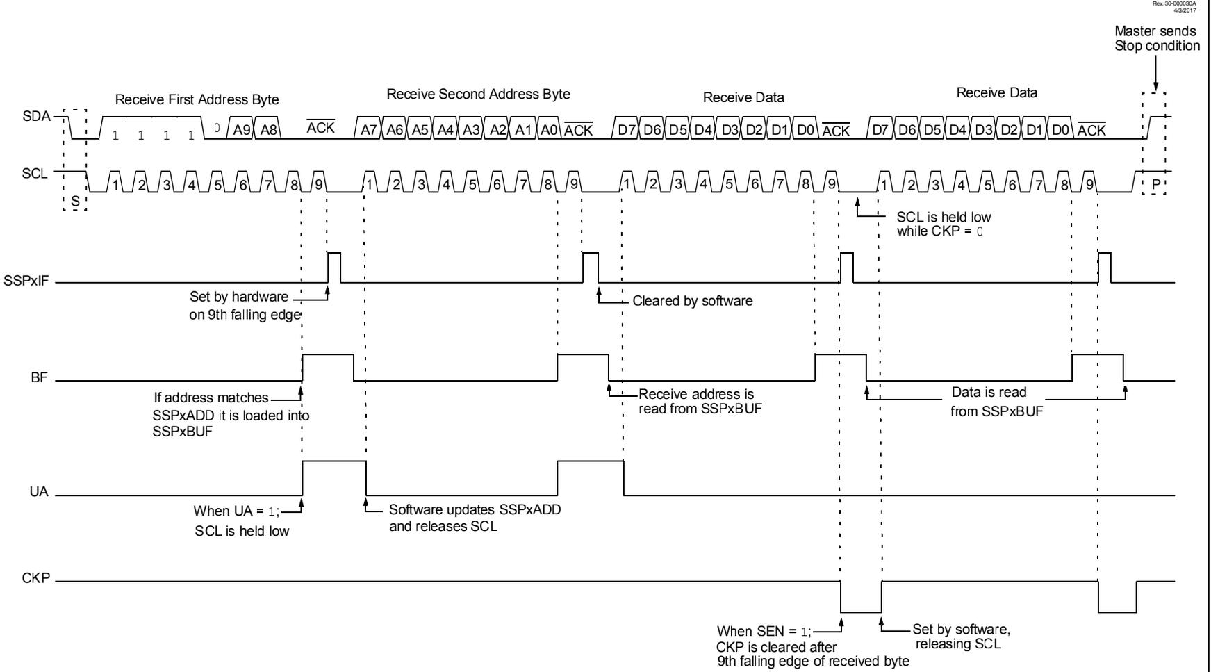
Figure 26-21. I<sup>2</sup>C Slave, 10-bit Address, Reception (SEN = 0, AHEN = 1, DHEN = 0)
