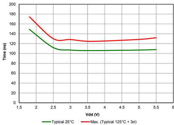
**Figure 39-28. Comparator Response Time Rising edge**
