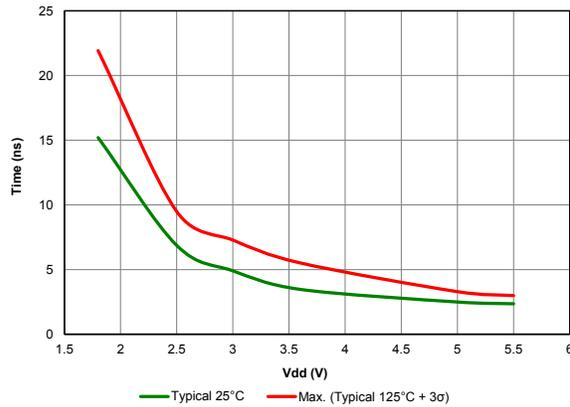
Figure 39-35. Fall time, slew rate control disabled
