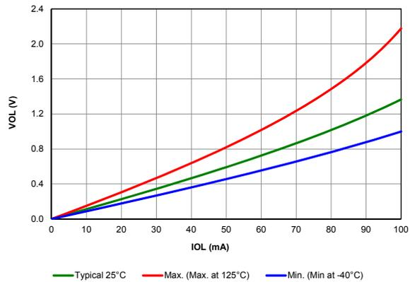
Figure 39-80. VOL vs. IOL OVER TEMPERATURE, VDD = 3V
