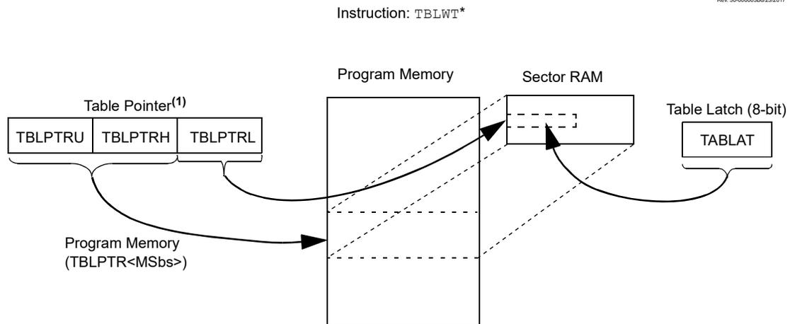
**Note 1:** During table writes the Table Pointer points to two areas. The LSbs of TBLPRTL point to an address within the sector RAM space. The MSbs of the Table Pointer determine where the sector will eventually be written.
