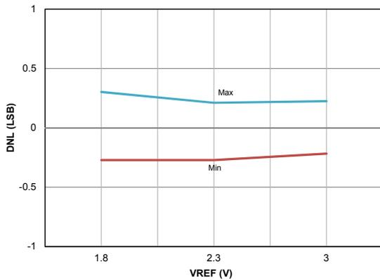
Figure 39-10. ADC 10-BIT, INL, Vdd = 3.0V, TAD = 1uS, Min and Max values at 125C + 3σ
