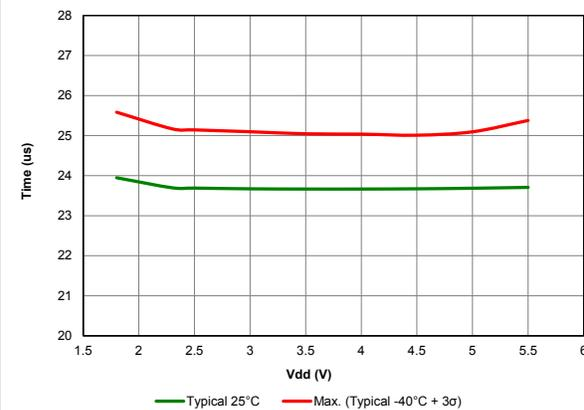
Figure 39-55. Wake From Sleep, VREGPM = 'b10, HFINTOSC = 16MHz
