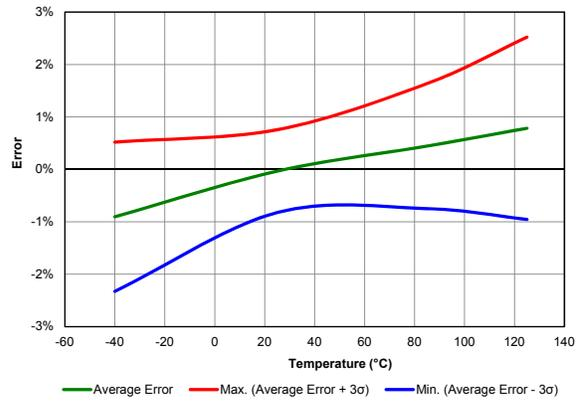
Figure 39-31. FVR Voltage Error 4x (Vdd = 5.5 V)
