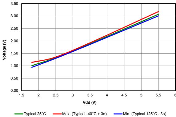
Figure 39-43. Schmitt Trigger Low Values
