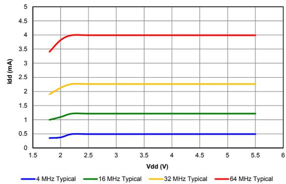
Figure 39-38. I<sub>DD</sub> MAXIMUM, INT Oscillator
