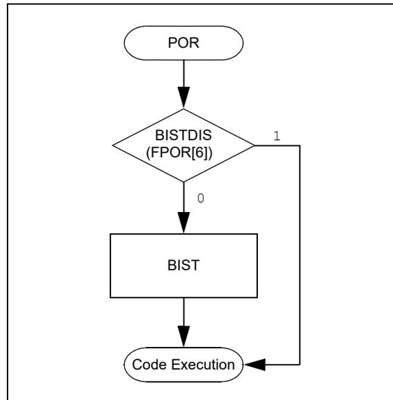
BIST will always run on FRC+PLL with PLL settings resulting in a 125 MHz clock rate. BIST at run time will use the same 125 MHz clock.
