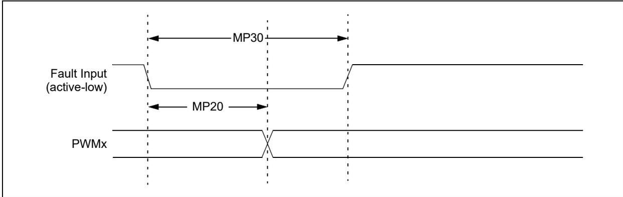
**FIGURE 24-6: HIGH-SPEED PWMx MODULE TIMING CHARACTERISTICS**
