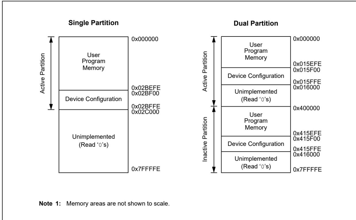
**FIGURE 3-5: PROGRAM MEMORY MAP FOR dsPIC33CH512MP50X/20X DEVICES<sup>(1)</sup>**
