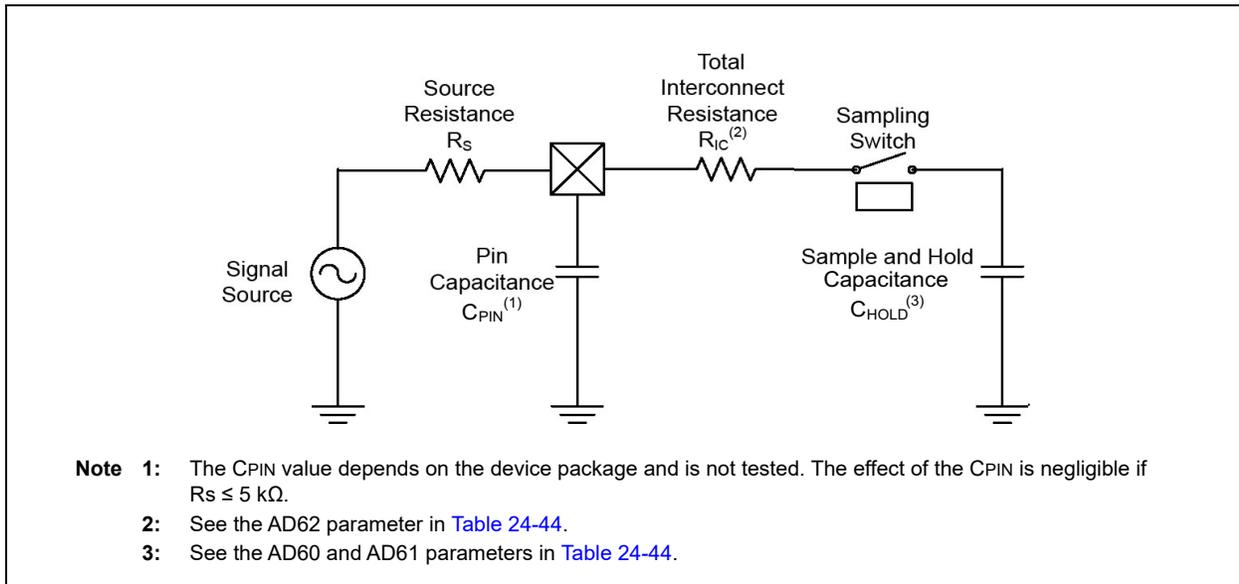
The total acquisition time for the Analog-to-Digital conversion is a function of the Holding Capacitor (CHOLD) charge time. For the ADC module to meet its specified accuracy, the Holding Capacitor (CHOLD) must be allowed to fully charge to the voltage level on the
