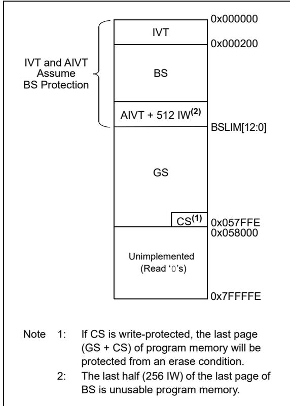
**FIGURE 21-6: MAIN FLASH SECURITY SEGMENTS (DUAL PARTITION MODE)**
