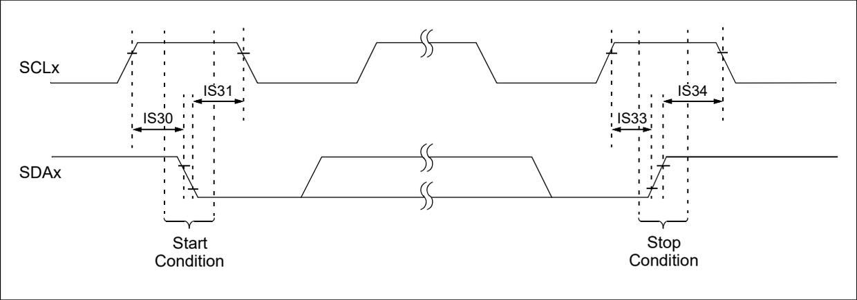
**FIGURE 24-16: I2Cx BUS DATA TIMING CHARACTERISTICS (CLIENT MODE)**
