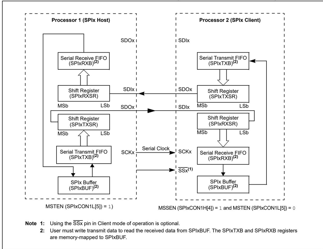
**FIGURE 14-5: SPIx HOST, FRAME HOST CONNECTION DIAGRAM**
