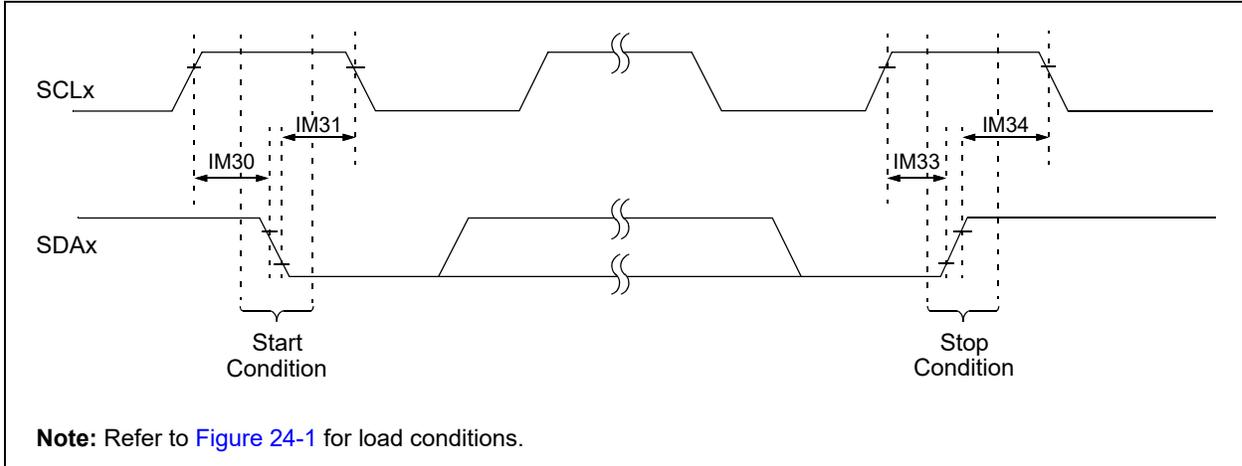
**FIGURE 24-14: I2Cx BUS DATA TIMING CHARACTERISTICS (HOST MODE)**
