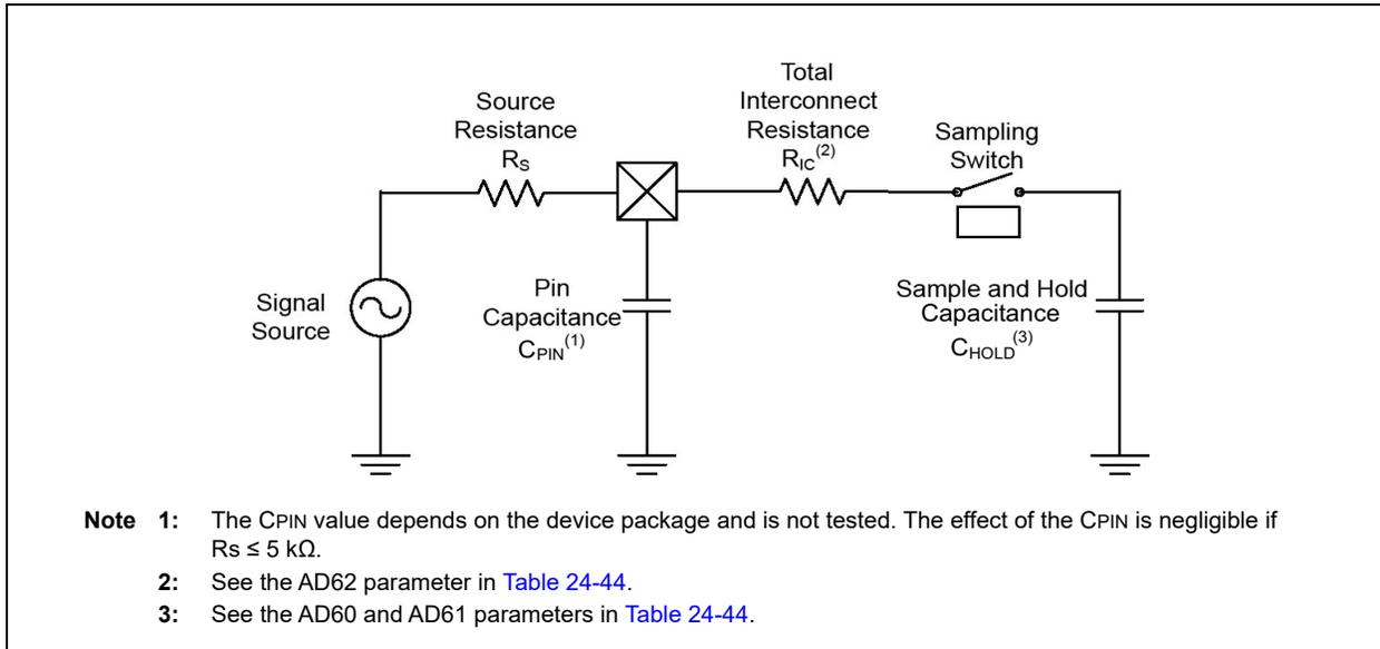
The total acquisition time for the Analog-to-Digital conversion is a function of the Holding Capacitor ( $C_{HOLD}$ ) charge time. For the ADC module to meet its specified accuracy, the Holding Capacitor ( $C_{HOLD}$ ) must be allowed to fully charge to the voltage level on the analog input pin. The Signal Source Impedance ( $R_S$ ) and the Interconnect Impedance ( $R_{IC}$ ) combine to
