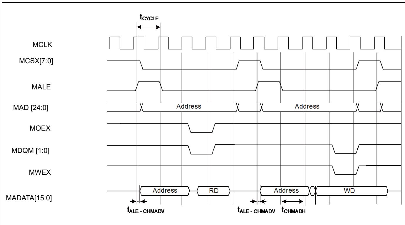
**Multiplexed Bus Access Synchronous SRAM Mode**
