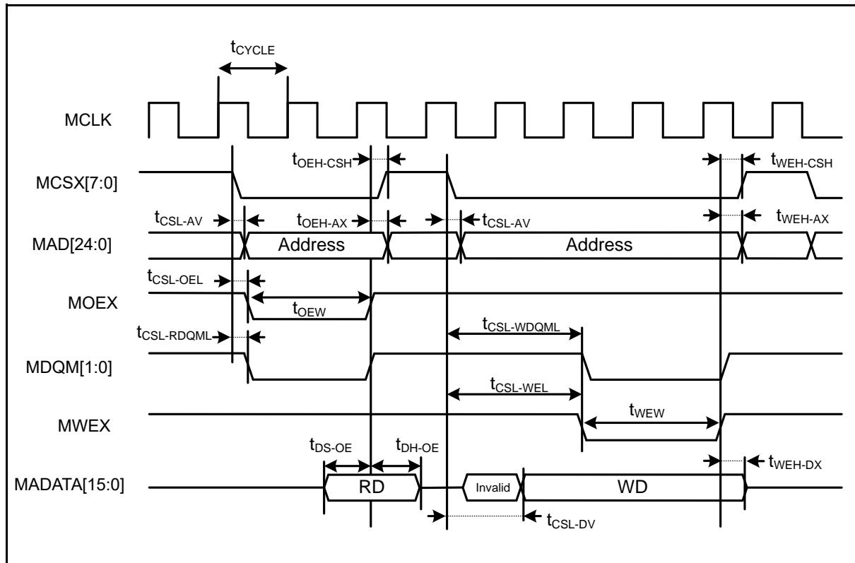
**Multiplexed Bus Access Asynchronous SRAM Mode**
