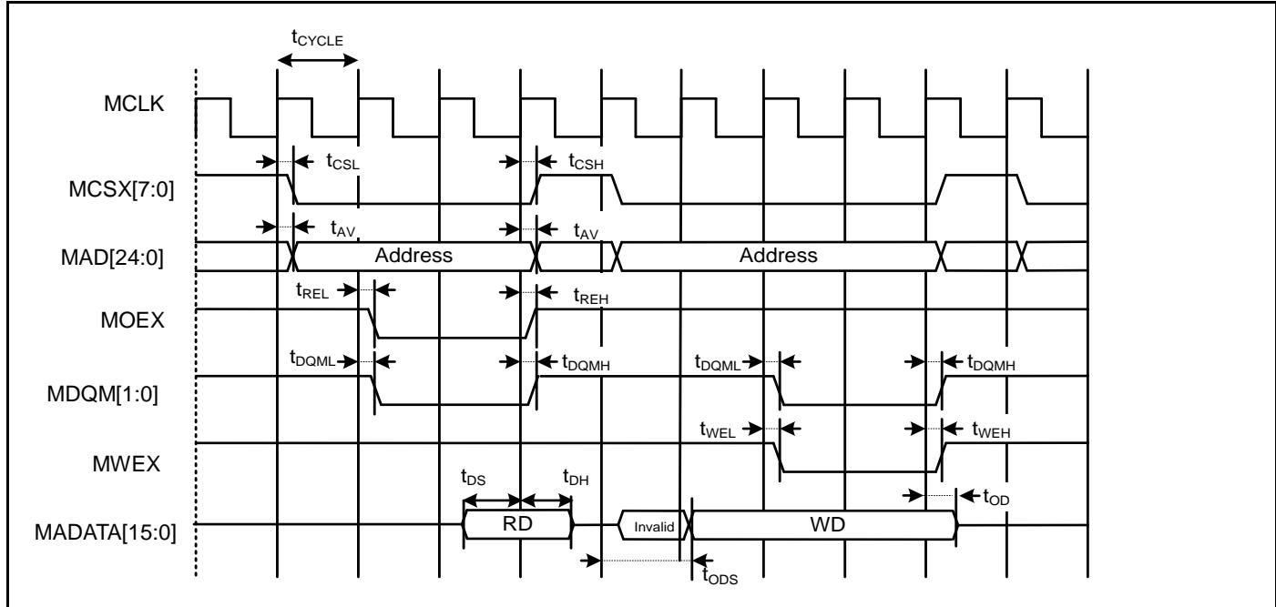
**Multiplexed Bus Access Asynchronous SRAM Mode**
