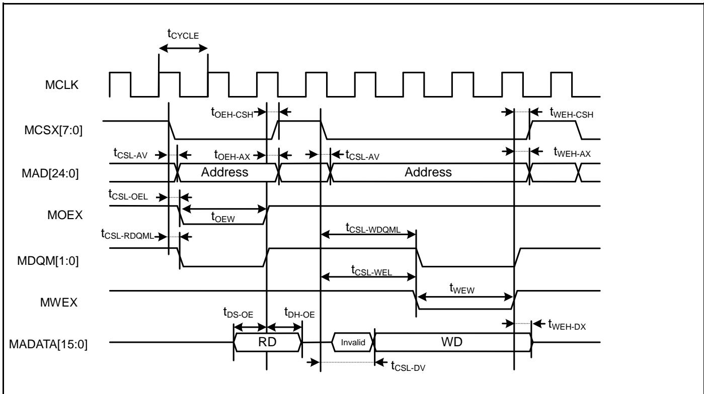
**Separate Bus Access Synchronous SRAM Mode**
