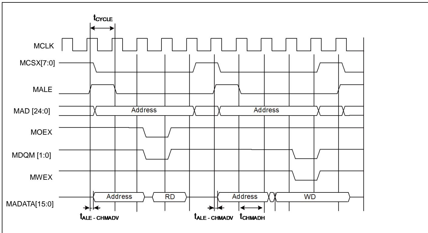
**Multiplexed Bus Access Synchronous SRAM Mode**
