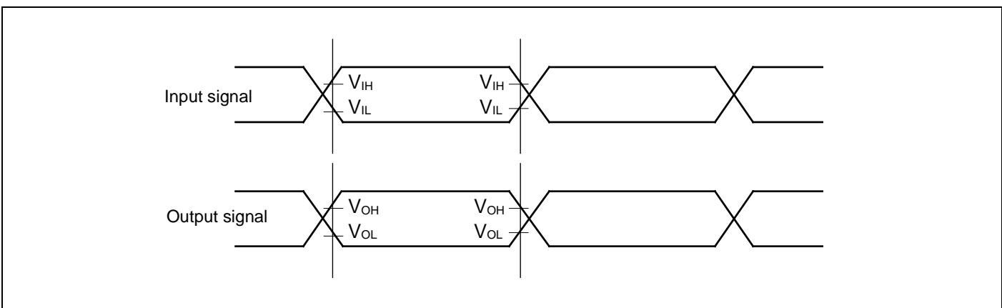
**Separate Bus Access Asynchronous SRAM Mode**
