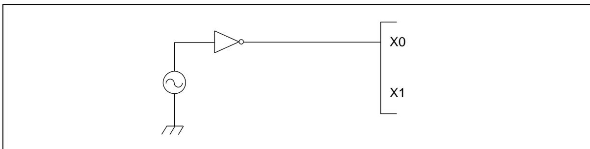
**13.3.2 Single Phase External Clock for Sub Oscillator**
