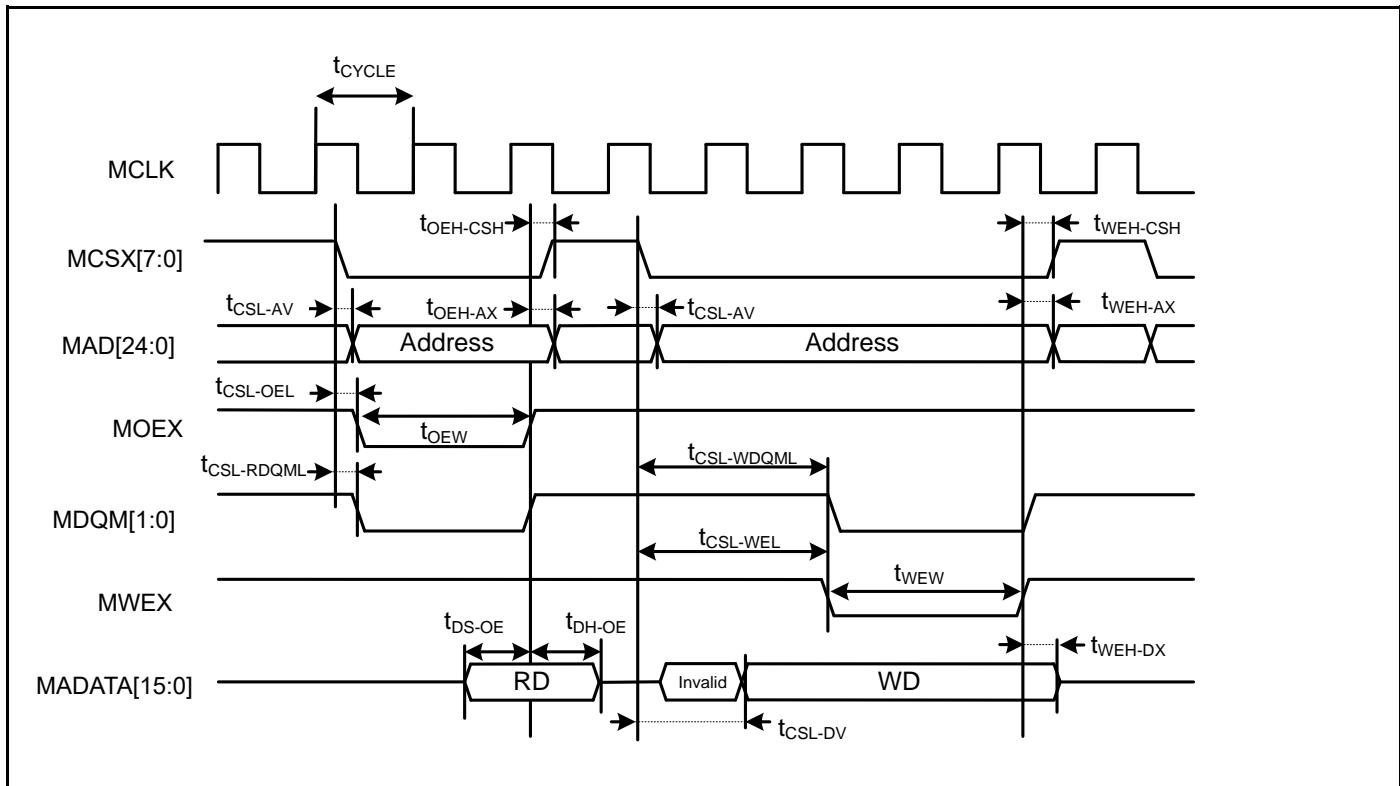
**Separate bus access synchronous SRAM mode**
