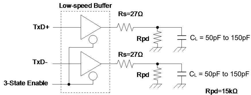
**Low-speed load (downstream port load) - Reference 2**
