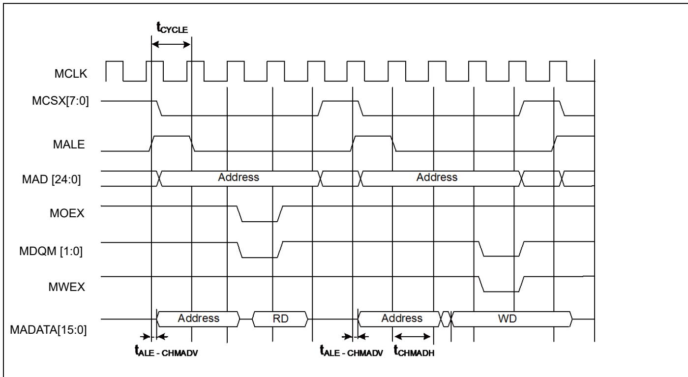
**Multiplexed bus access synchronous SRAM mode**
