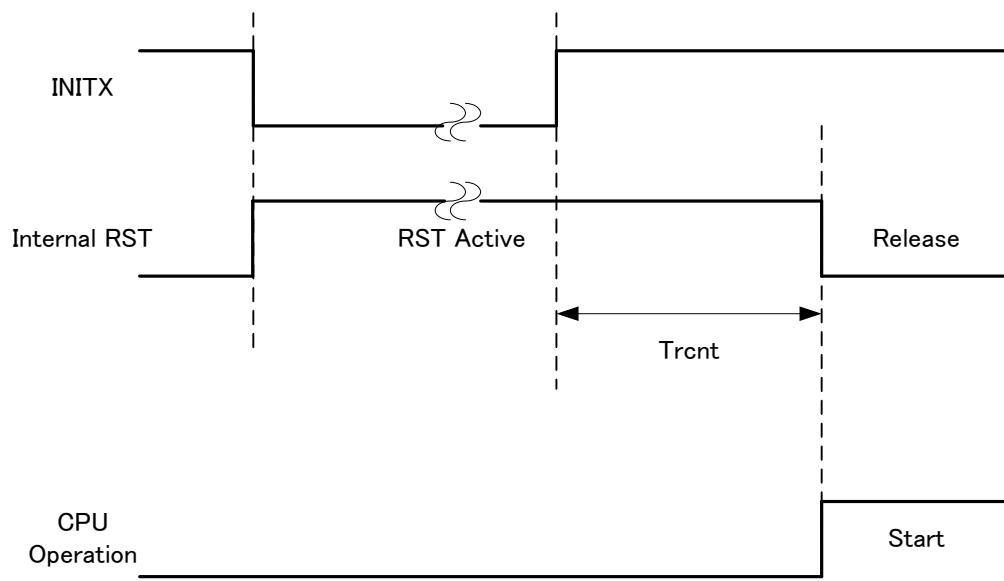
**Operation example of return from low power consumption mode (by internal resource reset<sup>\*1</sup>)**
