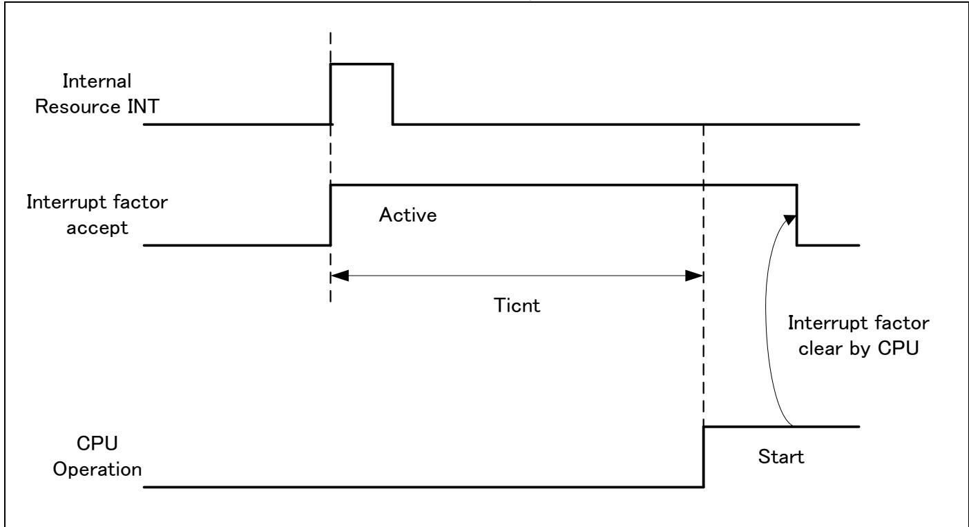
\*1: Internal resource interrupt is not included in return factor by the kind of Low-Power consumption mode.
