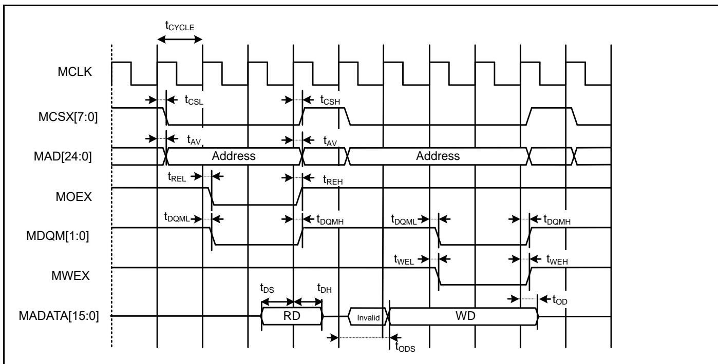
**Multiplexed bus access asynchronous SRAM mode**
