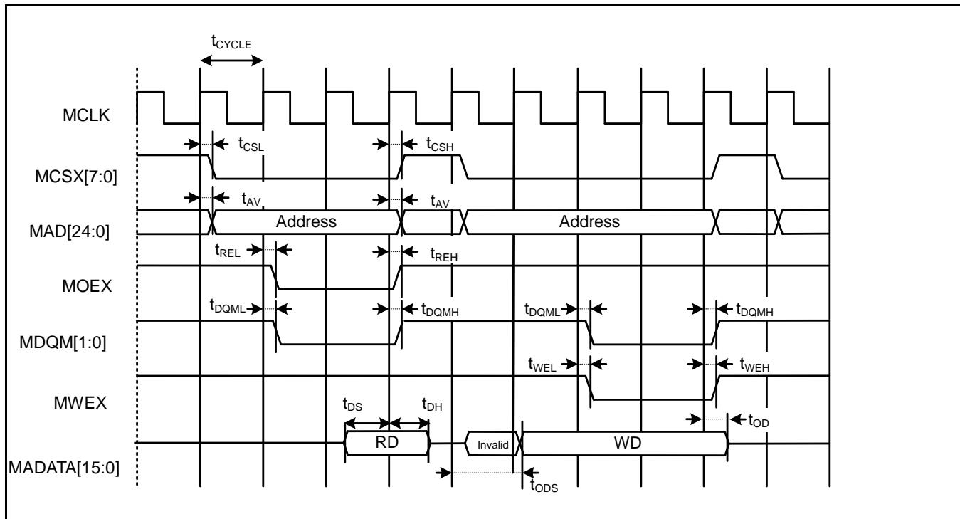
**Multiplexed Bus Access Asynchronous SRAM Mode**
