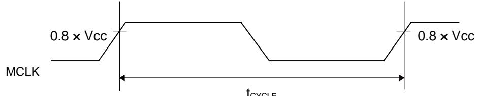
**External Bus Signal Input/output Characteristics**
