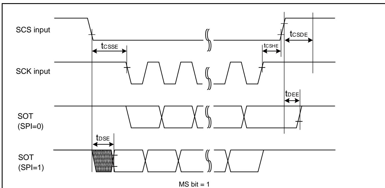
**When Using Synchronous Serial Chip Select (SCINV = 1, CSLVL=1)**
