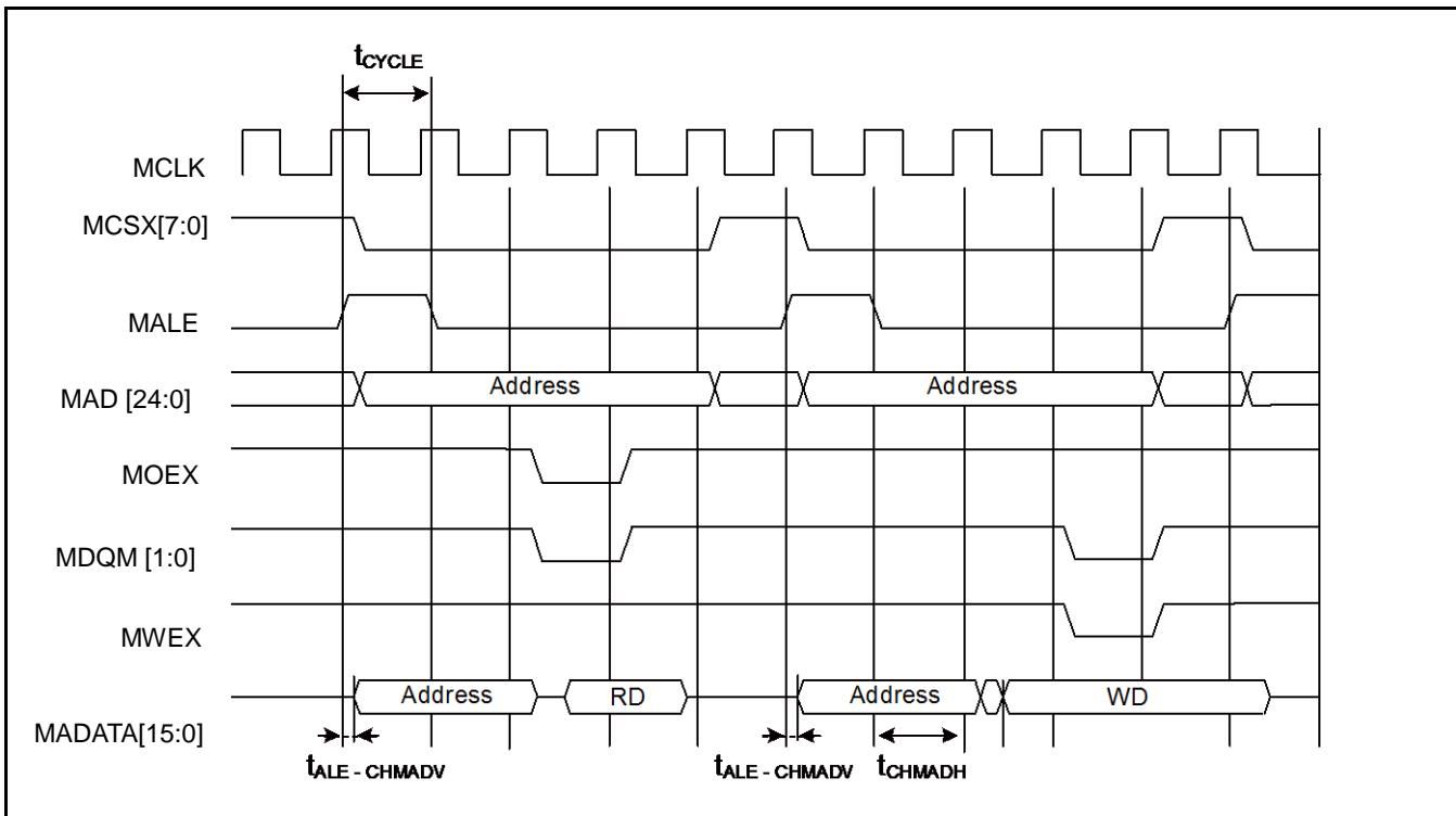
**Multiplexed Bus Access Synchronous SRAM Mode**
