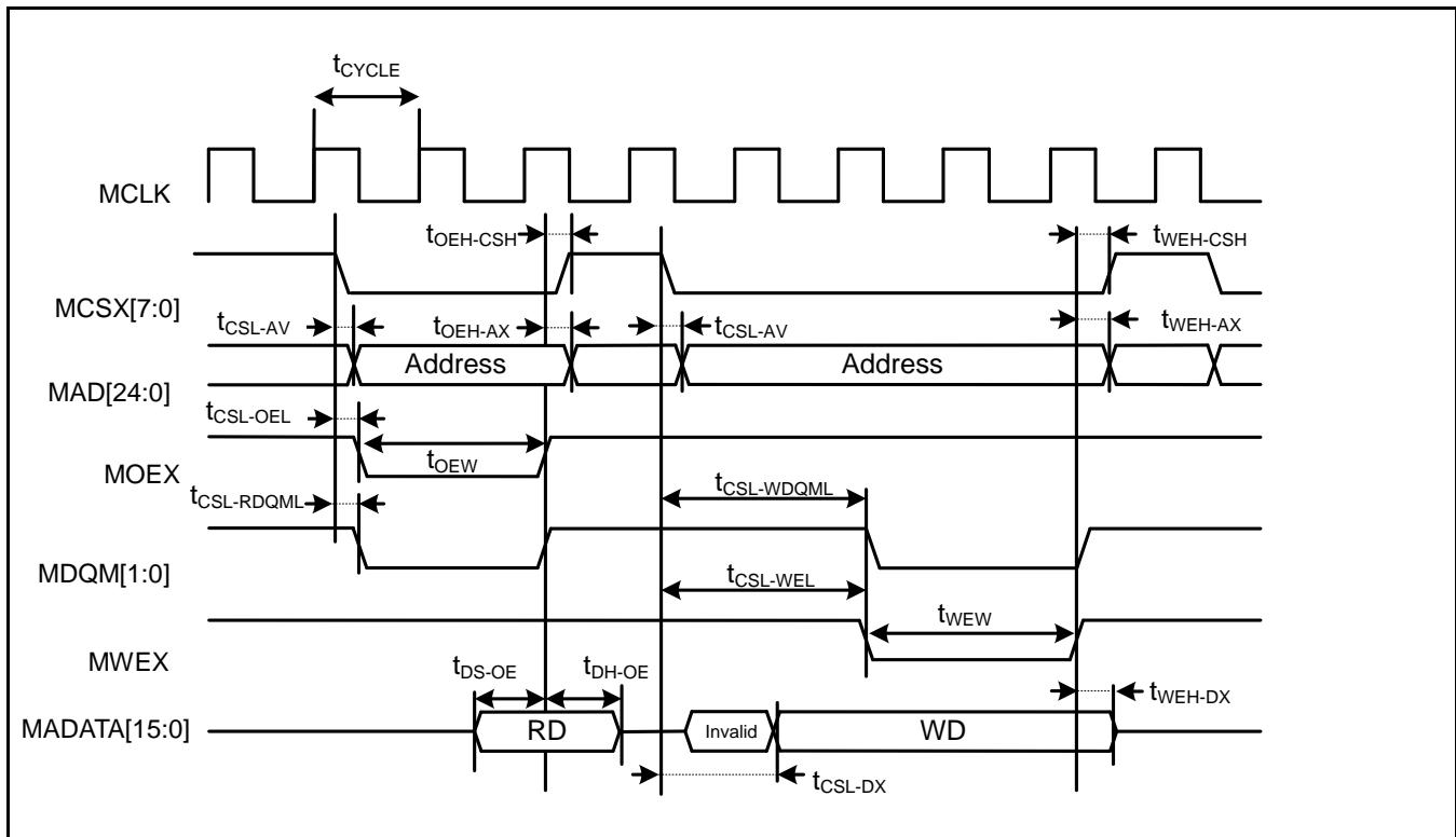
**Separate Bus Access Synchronous SRAM Mode**
