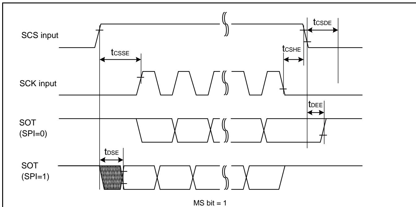
**High-speed Synchronous Serial (SPI = 0, SCINV = 0)**
