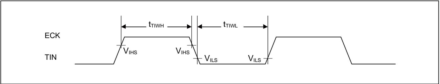
**Trigger input timing**
