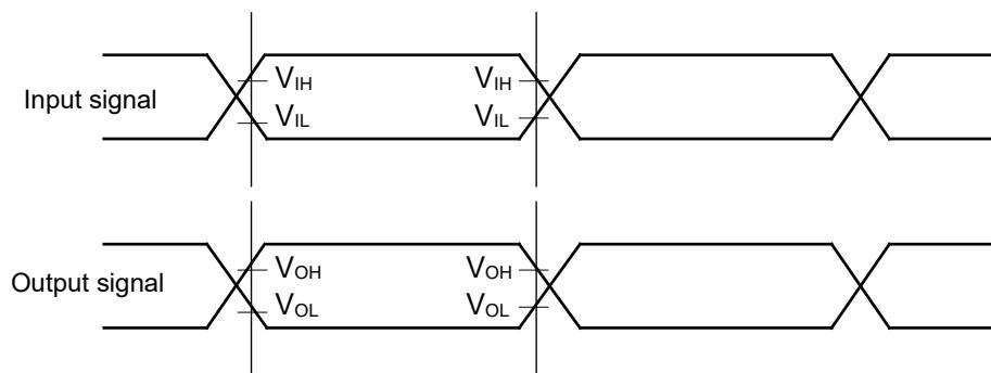
**Separate Bus Access Asynchronous SRAM Mode**
