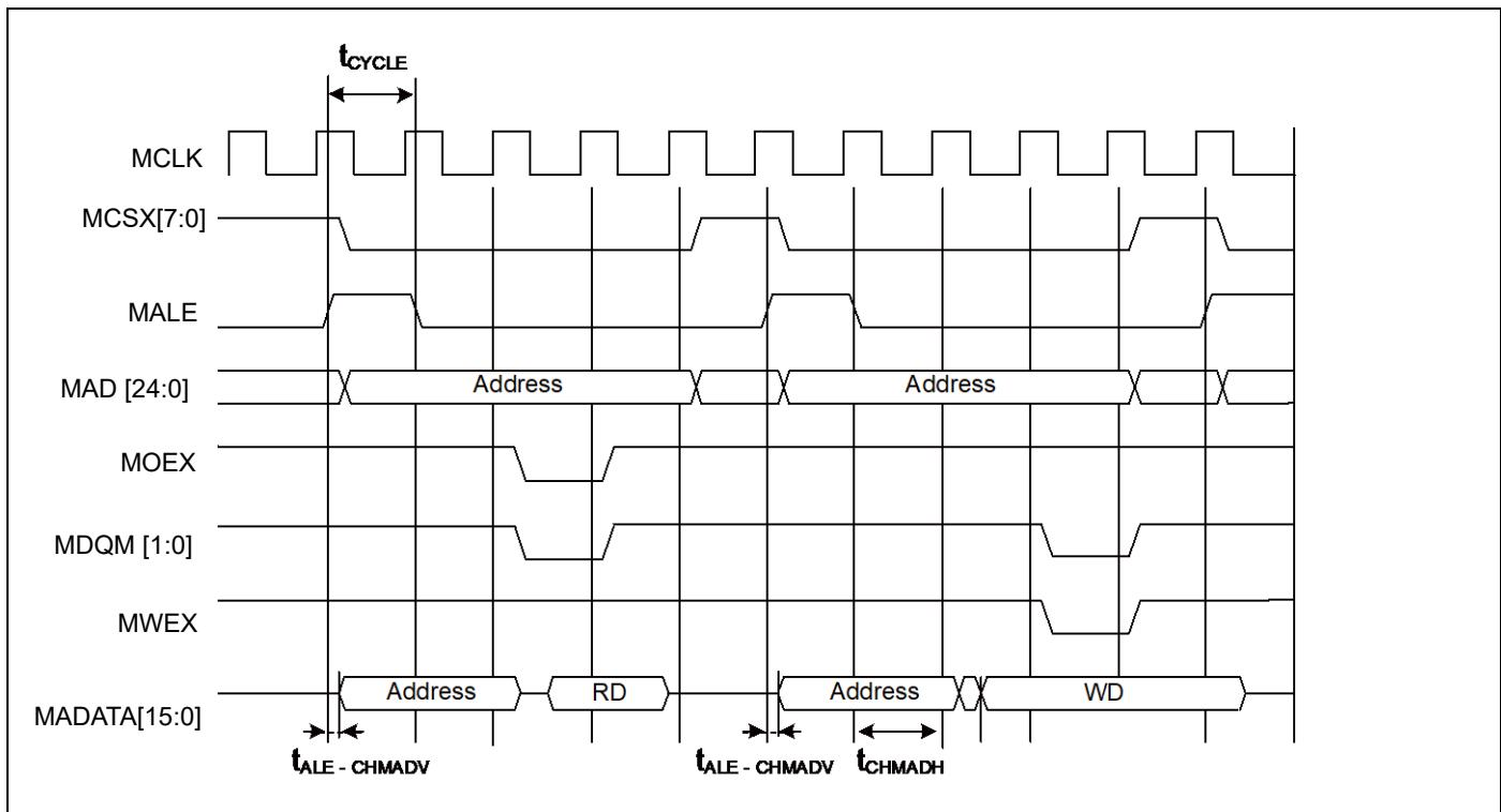
**Multiplexed Bus Access Synchronous SRAM Mode**
