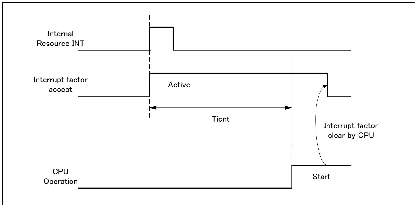
\*: Internal resource interrupt is not included in return factor by the kind of Low-Power consumption mode.
