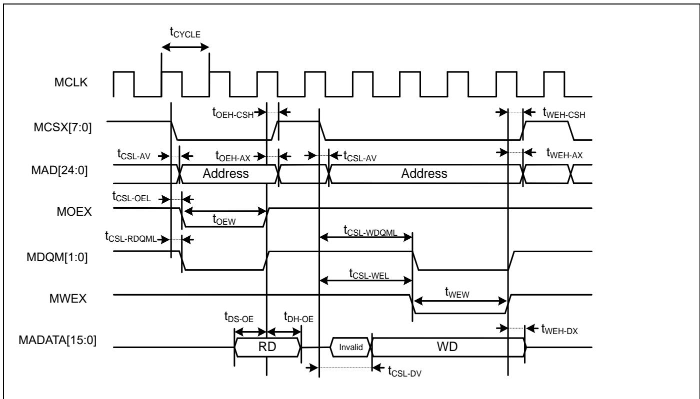
**Separate Bus Access Synchronous SRAM Mode**
