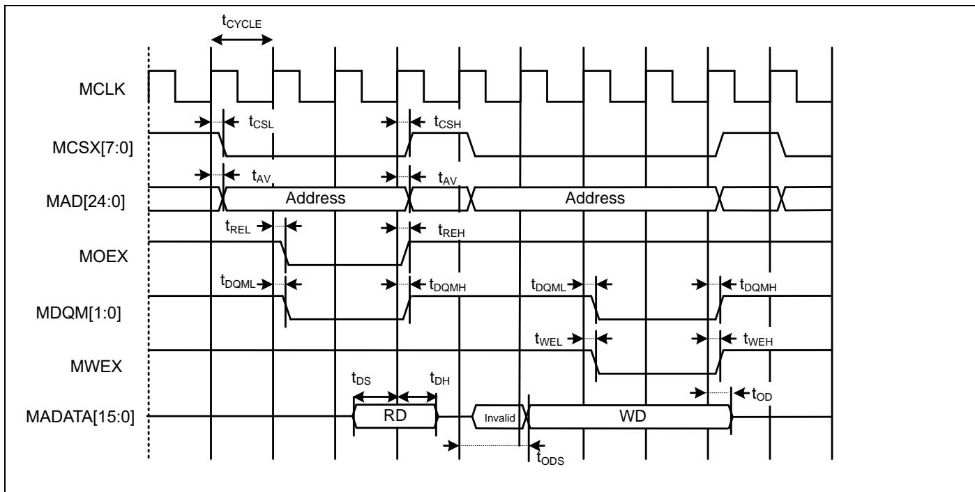
**Multiplexed Bus Access Asynchronous SRAM Mode**
