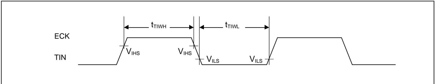
**Trigger input timing**
