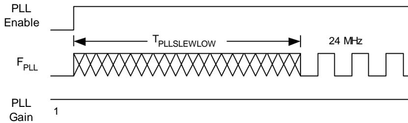
Figure 15. External Crystal Oscillator Startup Timing Diagram
