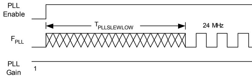
**Figure 11. External Crystal Oscillator Startup Timing Diagram**
