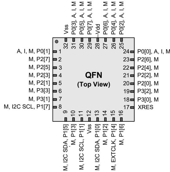
**Figure 10. CY8C21634 32-pin Sawn PSoC Device Sawn**
