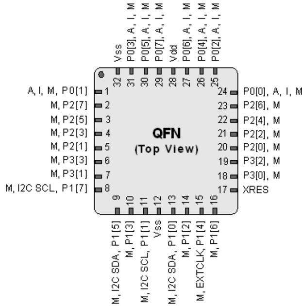
Figure 8. CY8C21634 32-pin PSoC Device
