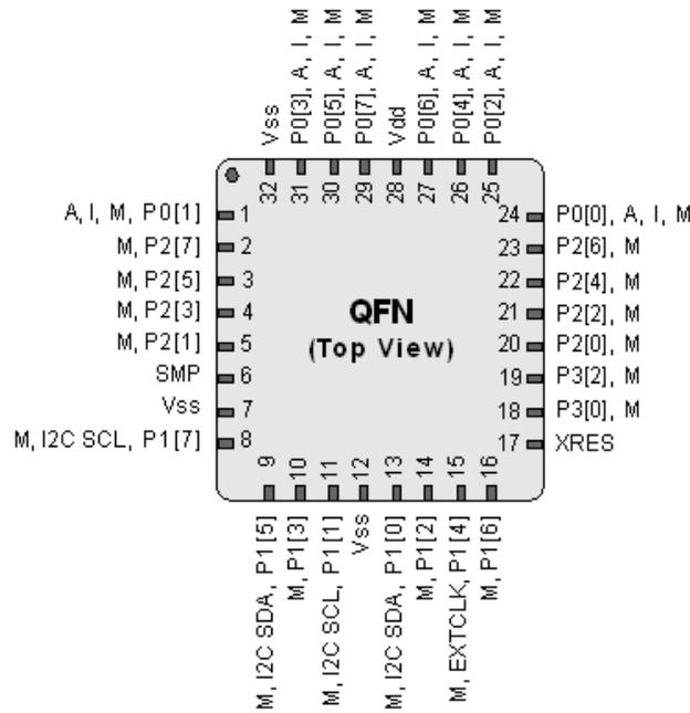
**Figure 9. CY8C21434 32-pin Sawn PSoC Device Sawn**
