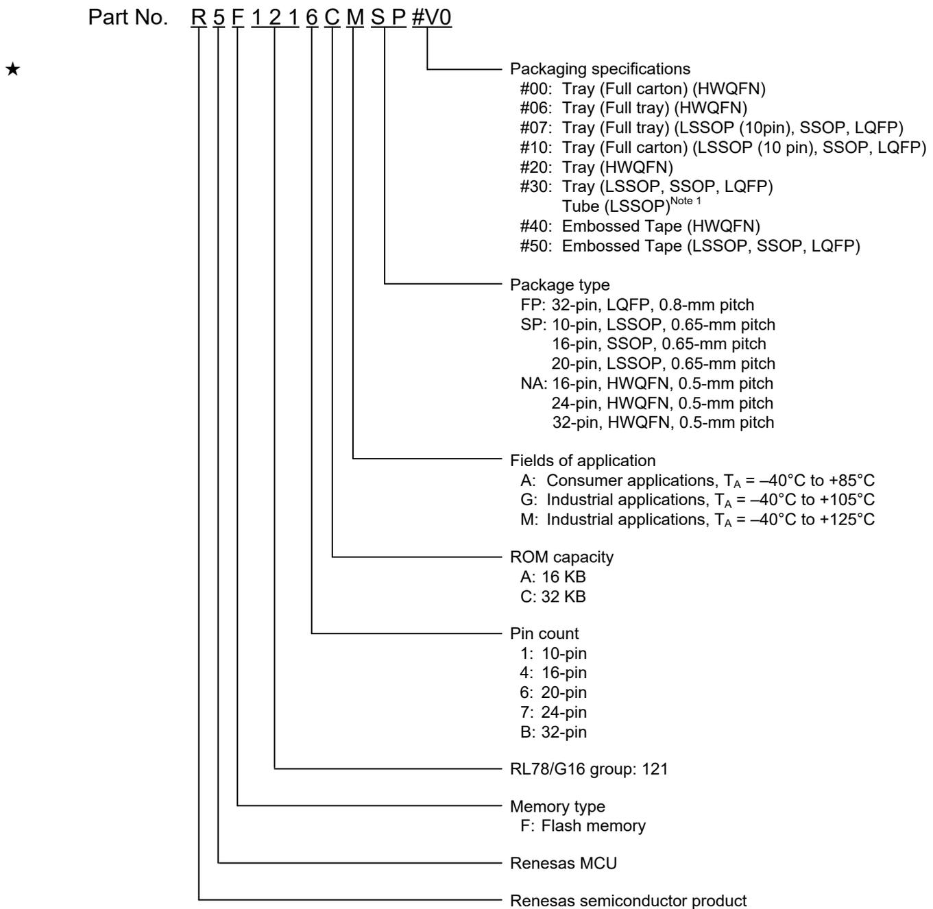
Note 1. For the 20-pin LSSOP products only, the packaging specification is Tube.
