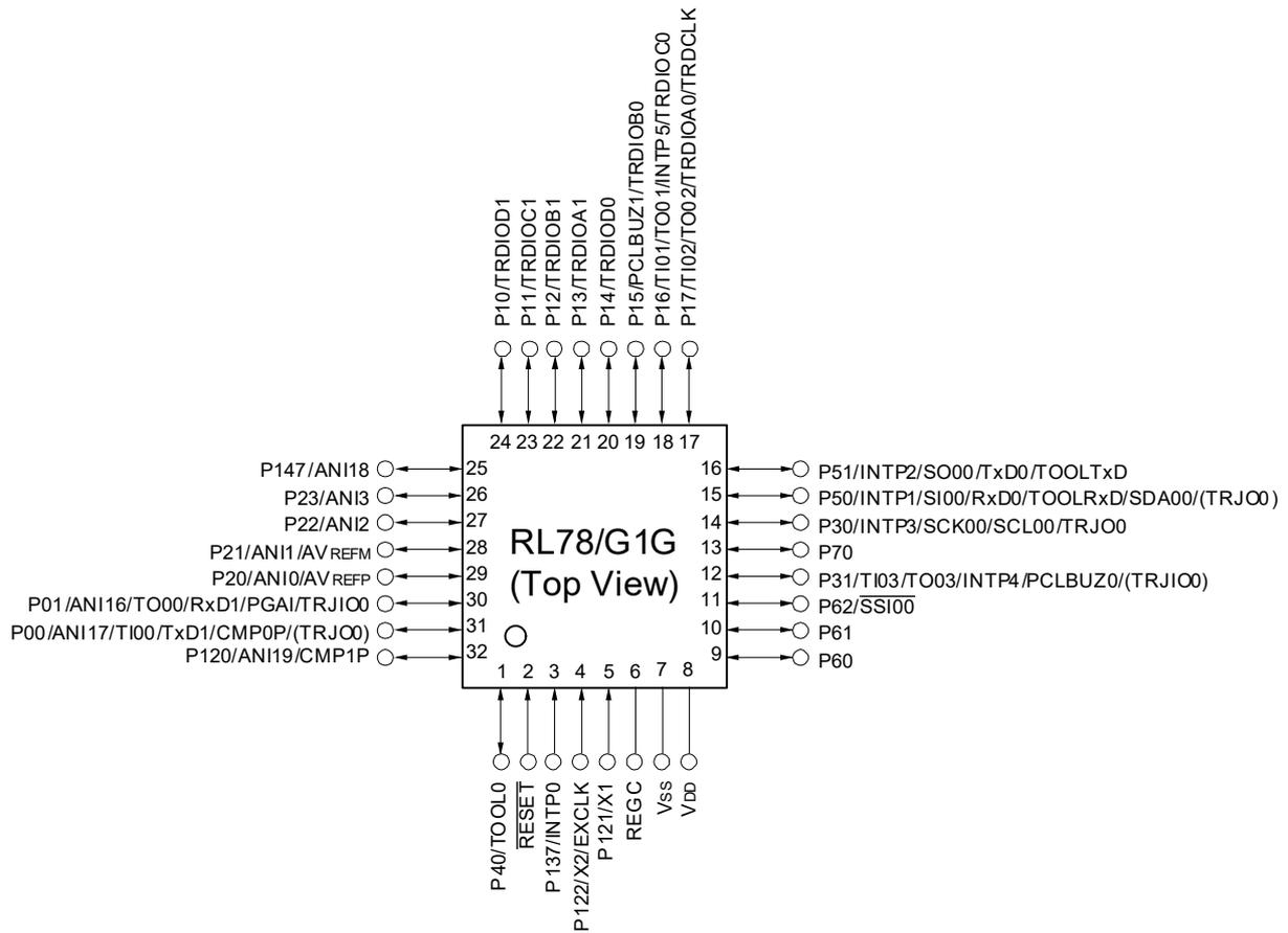
**Caution** Connect the REGC pin to Vss pin via a capacitor (0.47 to 1 μF).
