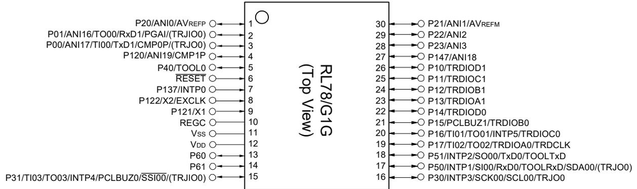
**Caution** Connect the REGC pin to V<sub>SS</sub> pin via a capacitor (0.47 to 1 μF).
