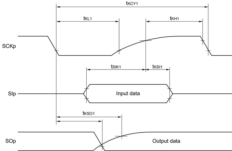
**Simplified SPI (CSI) mode serial transfer timing (master mode) (during communication at different potential)
