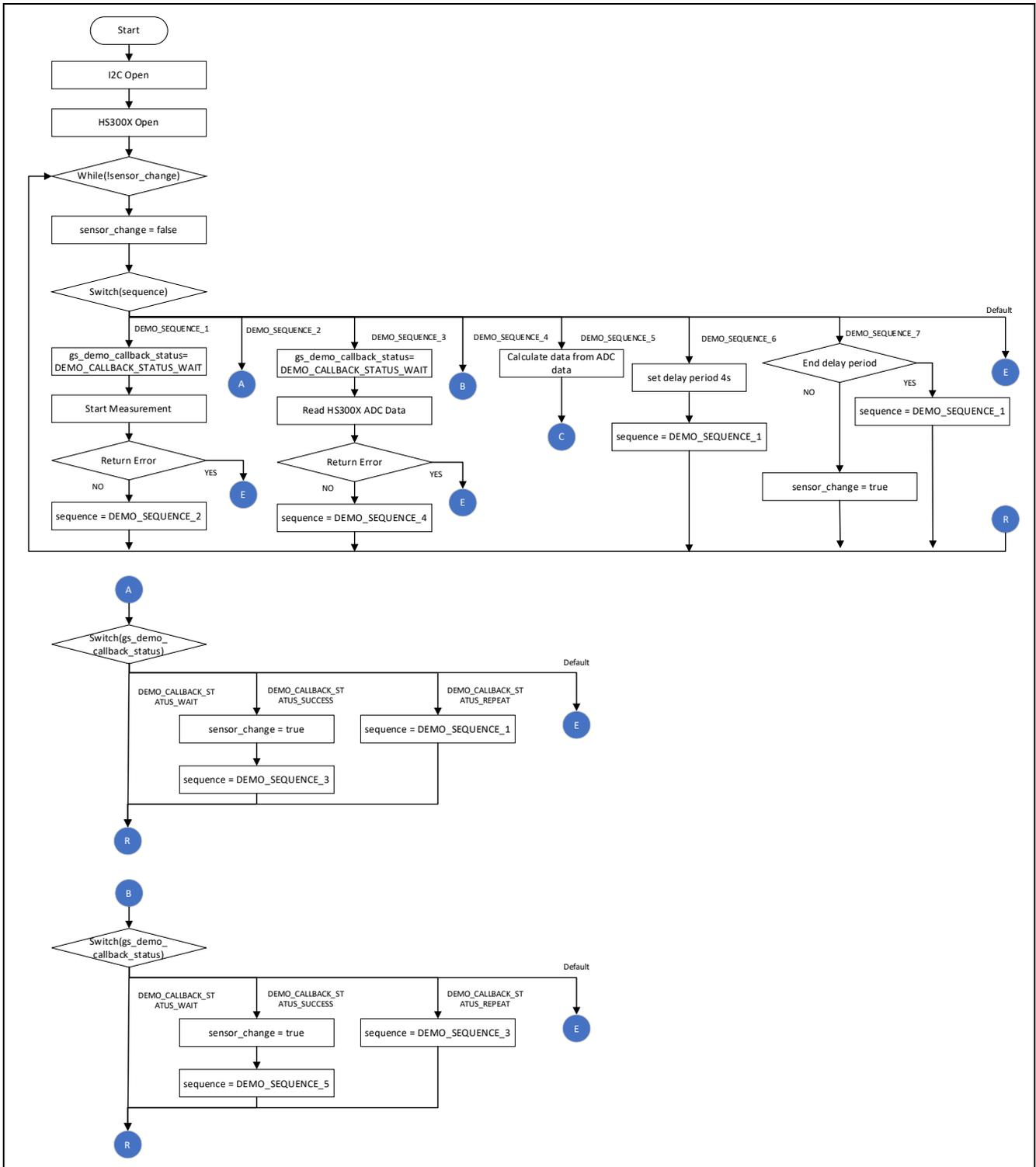
Figure 4-4 Flowchart of the Main Processing in the Non-OS Version of the Sample Software (1)
