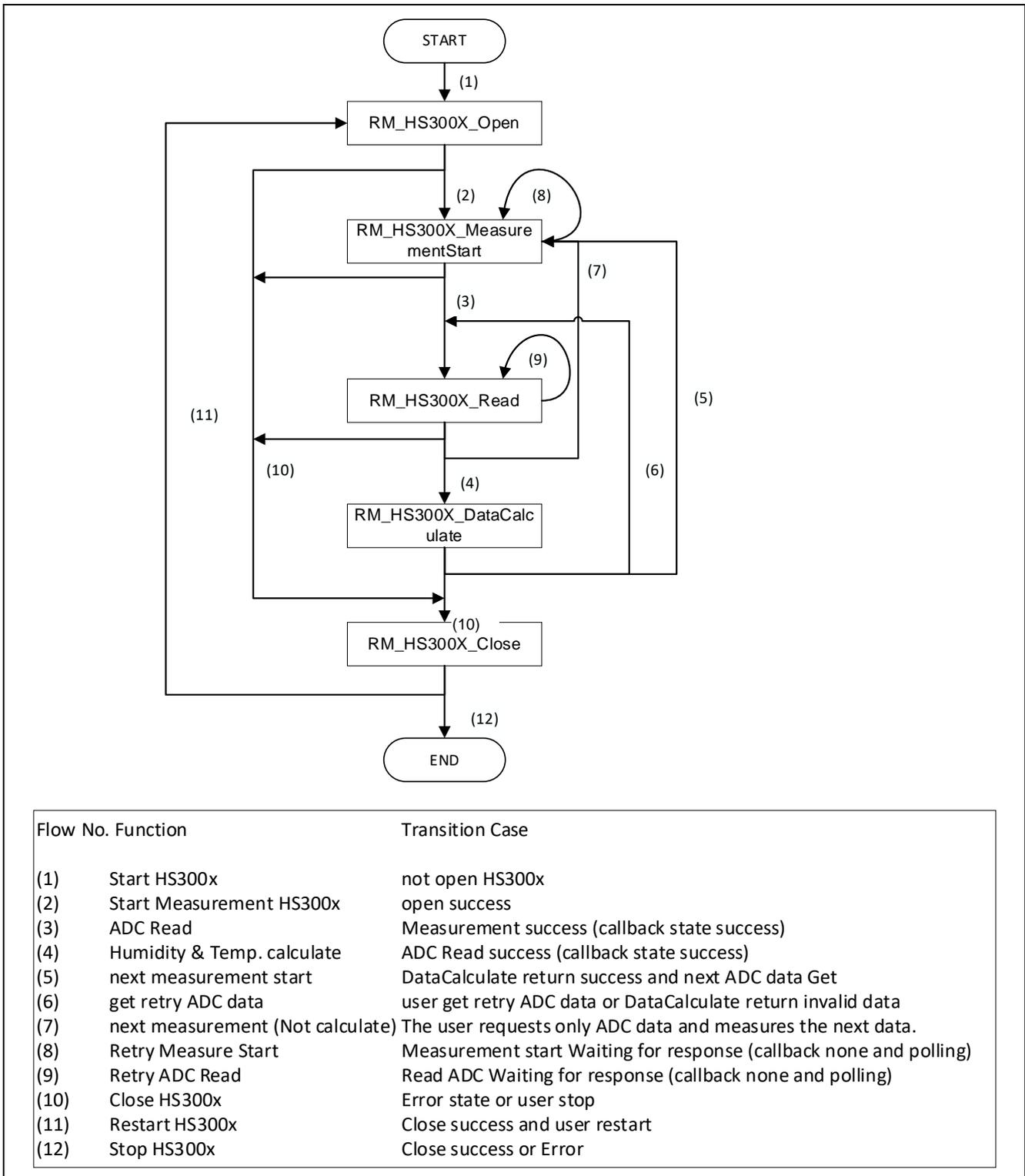
Figure 4-2 Diagram of Transitions between API Function Calls
