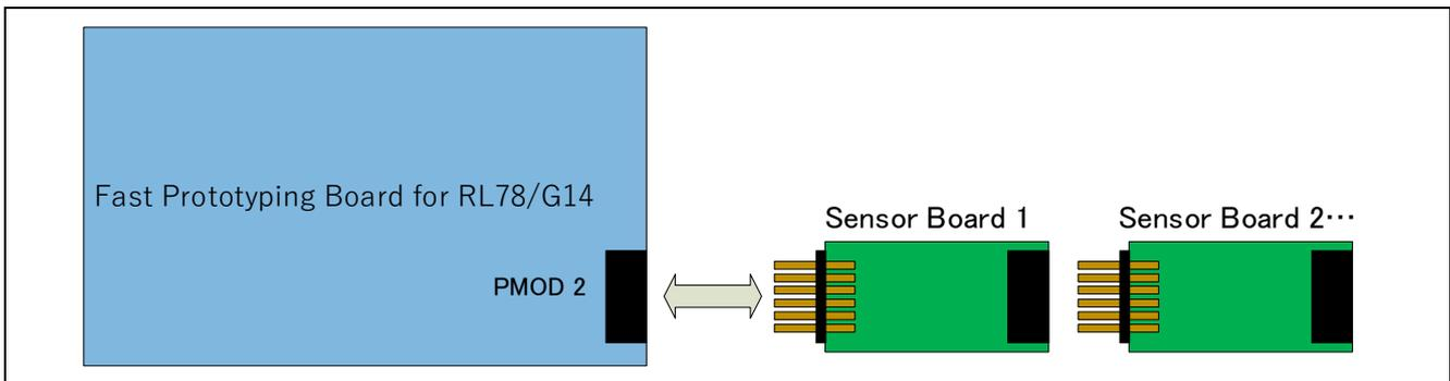
**Figure 2-3 Hardware Connections for the RL78/G14 Group**
