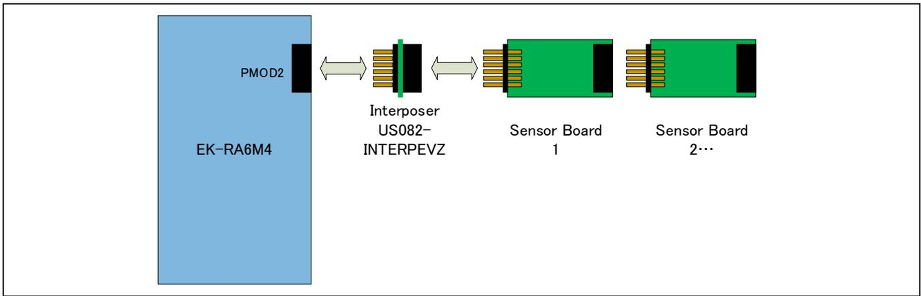
Figure 2-1 Hardware Connections for the RA Family
