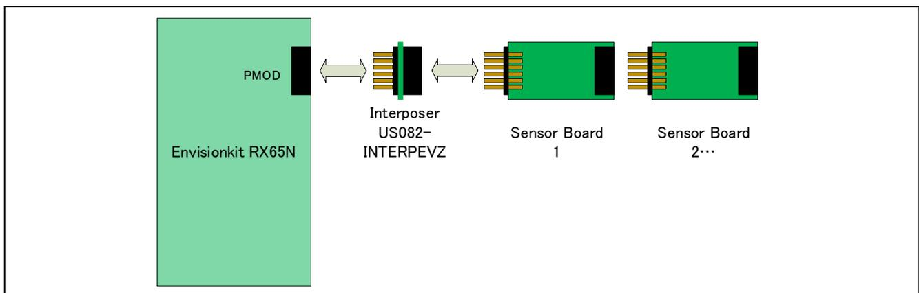
**Figure 2-2 Hardware Connections for the RX Family**
