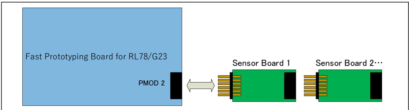
**Figure 2-4 Hardware Connections for the RL78/G23 Group**
