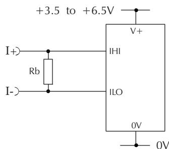
Measuring a current from a circuit which is floating with respect to the meter's supply, i.e. the current and the meter's power supply are isolated from each other.
