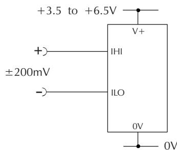
Measuring an input voltage referenced to a floating supply, i.e. the input voltage and the meter's power supply are isolated from each other.
